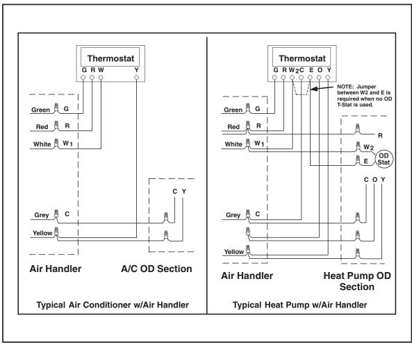
Figure 2. Typical Air Conditioning and Heat Pump System Connections
