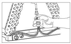
Figure 11. Restrictor Insertion in Distributor Body
