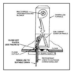
Figure 7. Downflow Furnace with Coil Cabinet
