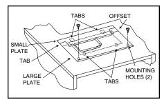
Figure 4. Close-Off Plates for Opening at Top of Furnace
