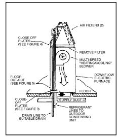
Figure 2. Downflow Furnace without Coil
