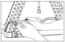
Figure 10. Removal of Orifice
