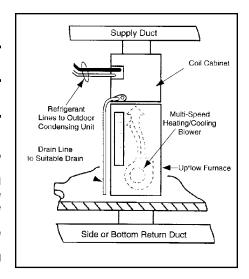
Figure 1. Upflow Furnace/Air Handler
