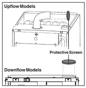
Figure 4. Protective Screen for One Pipe Installations
