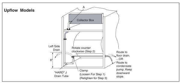
Figure 18. Furnace with Condensate Drain Trap Assembly
