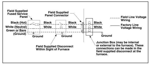
Figure 21. Line Voltage Field Wiring
