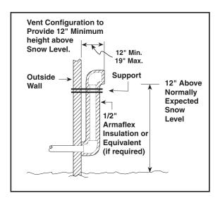
Figure 15. Alternate Horizontal Vent Installation
