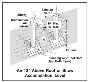
Figure 17. Vertical Vent Termination
