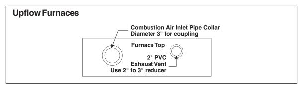
Figure 12. Furnace Pipe Adaptions
