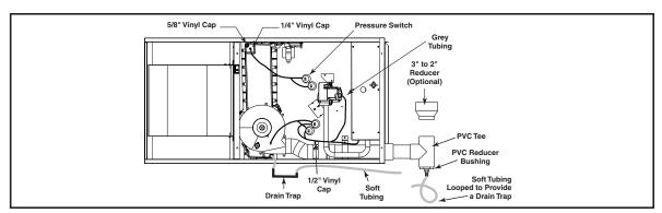
Figure 2. 90+ Upflow Converted for Horizontal Installation (Horizontal Right)
