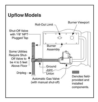
Figure 19. Typical Gas Service Connection
