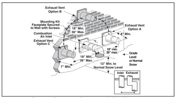
Figure 16. Exhaust and Combustion Air Pipe Clearances
