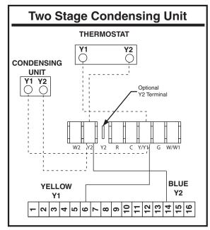
Figure 28. Two Stage Condensing Unit
