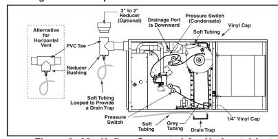
**NOTE:** When converting the furnace, to horizontal left, ensure that the drainage port on the in-line drain assembly is downward as shown in this figure. If the in-line drain assembly is not rotated, then the furnace may not drain properly.
