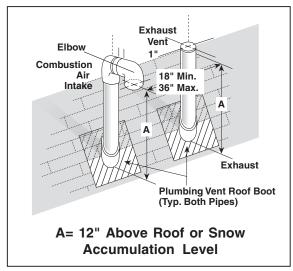
Figure 22. Vertical Vent Termination
