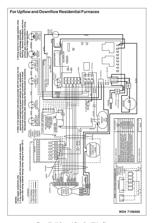
Figure 28. Upflow and Downflow Wiring Diagram
