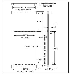
Figure 9. Downflow Sub-Base Dimensions
