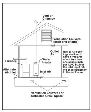
Figure 14. Equipment in a Confined Space with all Combustion Air drawn from Outdoors through Ventilated Crawl Space and Ventilated Attic
