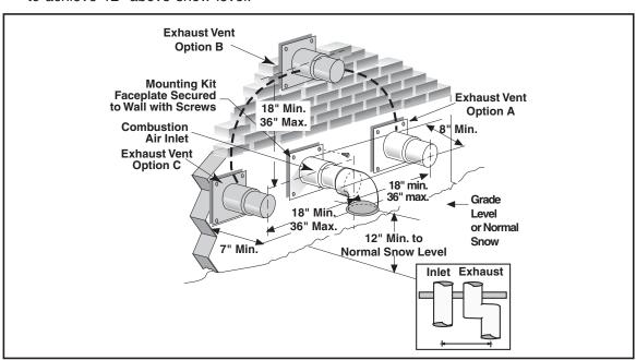
Figure 21. Exhaust and Combustion Air Pipe Clearances
