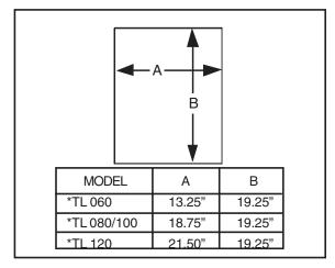
Figure 5. Opening for Concrete Slab
