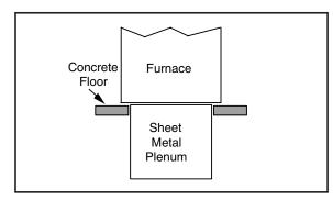
Figure 6. Downflow Furnace on a Concrete Slab
