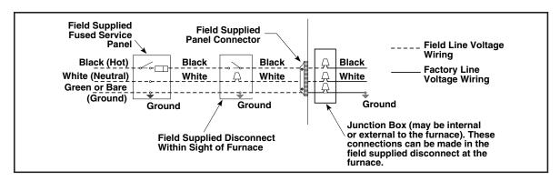
Figure 25. Line Voltage Field Wiring
