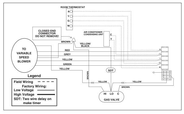
Figure 26e. Timed Two Stage Configuration
