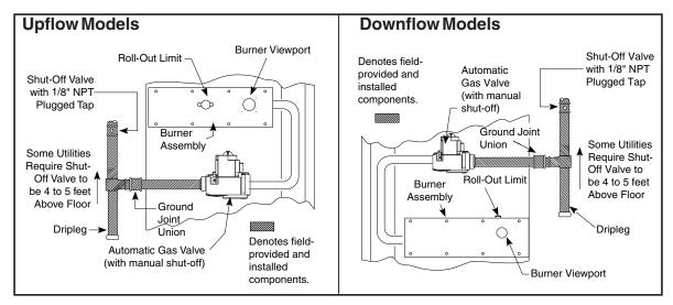
Figure 24a. Typical Gas Service Connection
