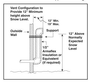
Figure 20. Alternate Horizontal Vent Installation
