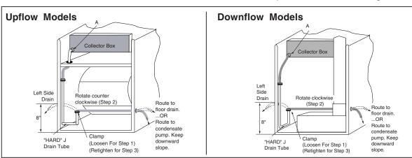
Figure 23. Furnace with Condensate Drain Trap Assembly
