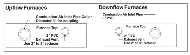
Figure 18. Furnace Pipe Adaptions
