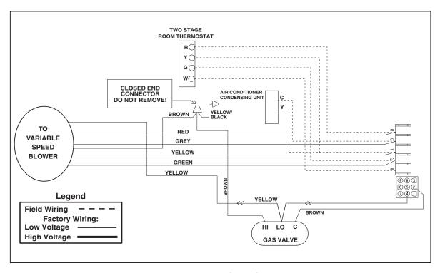
Figure 26c. Low Fire Only Configuration
