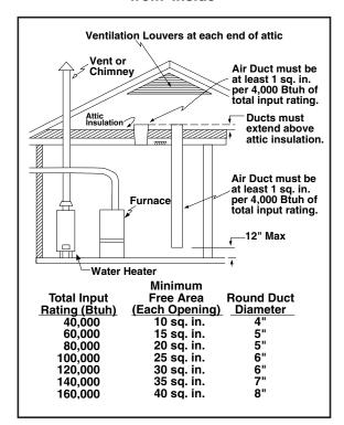
Figure 13. Equipment in a Confined Space with all Combustion Air drawn from Outdoors through Vertical Ducts – from Ventilated Attic
