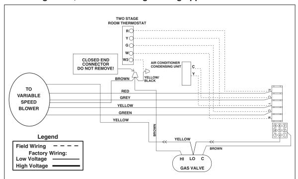
Figure 26a. Two Stage Configuration
