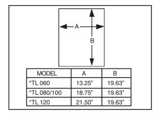
Figure 7. Opening in Wood Floor
