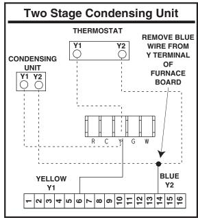
Figure 27. Two Stage Condensing Unit
