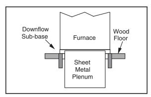
Figure 8. Furnace on a Wood Floor
