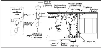
**NOTE:** When converting the furnace, to horizontal left, ensure that the drainage port on the in-line drain assembly is downward as shown in this figure. If the in-line drain assembly is not rotated, then the furnace may not drain properly.
