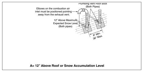
Figure 23. Vertical Vent Termination
