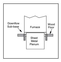
Figure 8. Furnace on a Wood Floor
