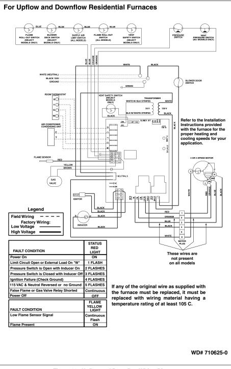
Figure 29. Upflow and Downflow Wiring Diagram
