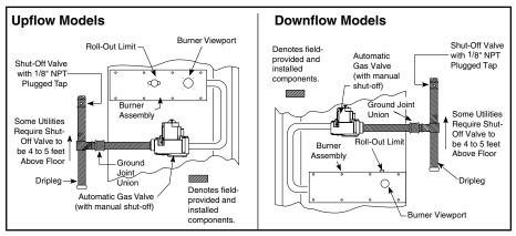
Figure 25. Typical Gas Service Connection
