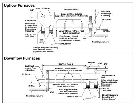
\* These neoprene couplings are field-supplied and can be used if the installation requires breakable connections in the piping. Note that a maximum of two couplings per pipe are allowed.
