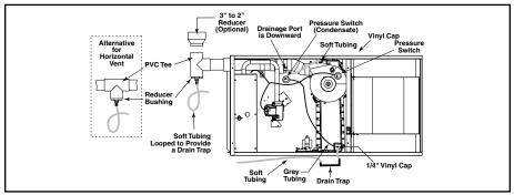
Figure 4. 90+ Upflow Converted for Horizontal Installation (Horizontal Left)
