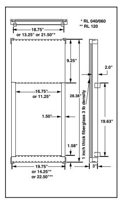
Figure 9. Downflow Sub-Base Dimensions
