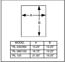
Figure 5. Opening for Concrete Slab
