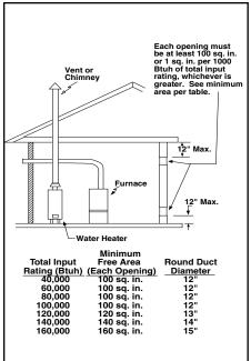
Figure 11. Equipment in a Confined Space with all Combustion Air drawn from Inside
