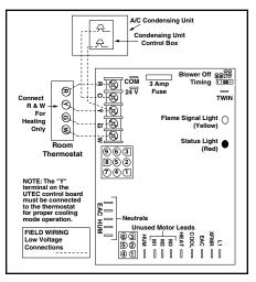
Figure 27. Low Voltage Field, Four-wire Heating/Cooling Applications
