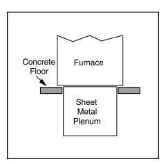
Figure 6. Furnace on a Concrete Slab
