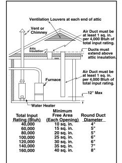
Figure 13. Equipment in a Confined Space with all Combustion Air drawn from Outdoors through Vertical Ducts – from Ventilated Attic
