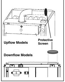
Figure 10. Protective Screen for One Pipe Installations
