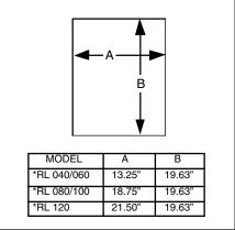
Figure 7. Opening in Wood Floor
