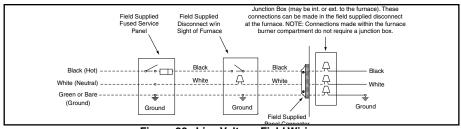
Figure 26. Line Voltage Field Wiring
