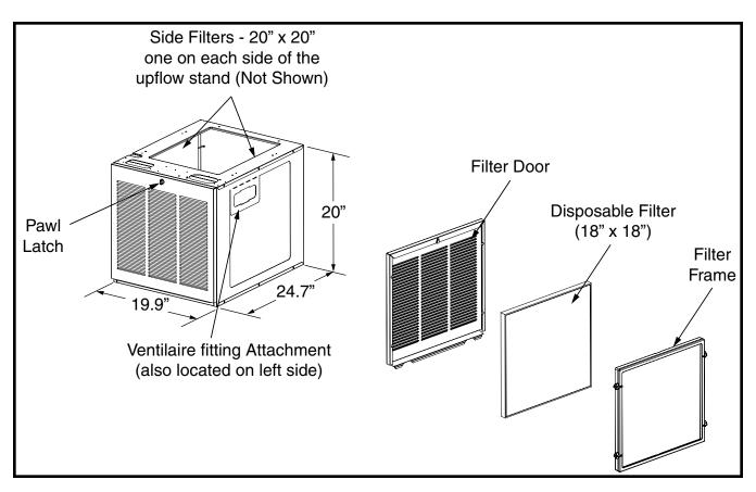
Figure 1. Upflow Stand for Electric Furnaces
