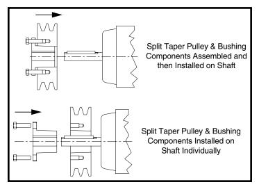
Figure 4. Split Taper Bushing & Pulley Assembly Options
