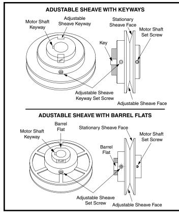
Figure 3. Adjustable Sheaves with Keyways or Barrel Flats
