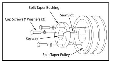
Figure 5. Split Taper Bushing & Pulley Assembly
