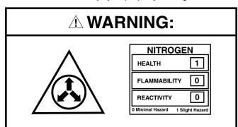
C6 coils are pressurized with nitrogen at the factory. Avoid direct face exposure or contact with valve when gas is escaping. Always ensure adequate ventilation is present during the depressurization process. Any uncertainties should be addressed before proceeding.
