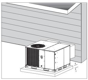
Figure 5. Ground Level Installation
