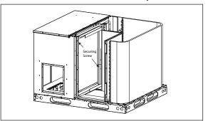
Figure 3a. Internal filter Rack Location
