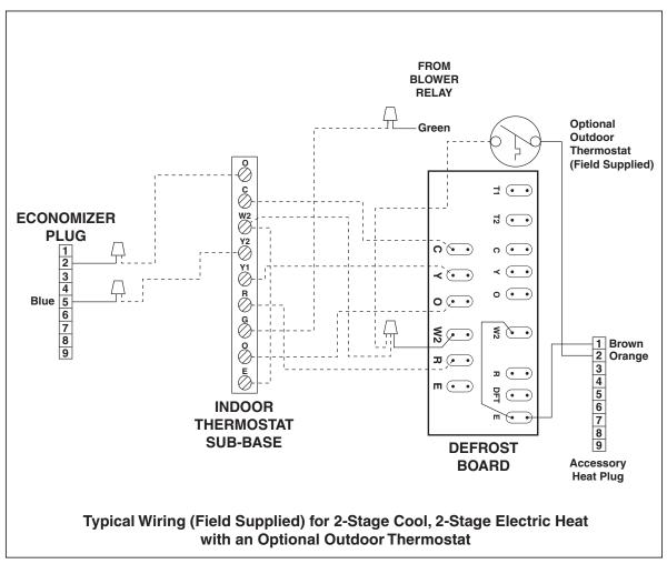
**Figure 8. Typical Heat Pump Thermostat Connections**
