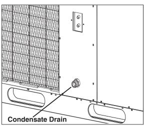
Figure 4. Condensate Drain
