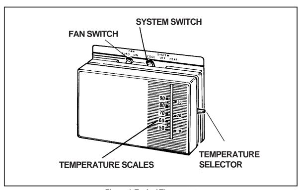
Figure 1. Typical Thermostat
