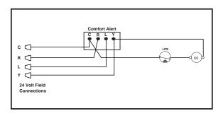
Figure 3. 24VAC Comfort Alert™ Wiring Diagram
