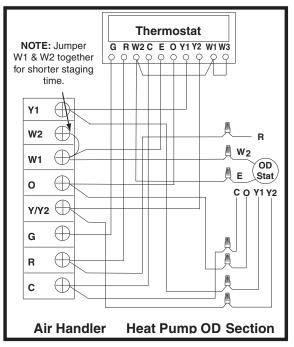
Figure 2. Typical 2 - Stage Heat Pump w/ Optional Outdoor Thermostat and Variable Speed Air Handler
