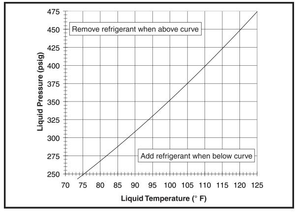
Figure 4. Charging Chart for 2 Ton Units
