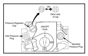
Figure 35. Gas Valve - Top View
