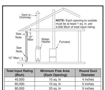
Figure 5. Combustion Air Drawn from Outside Through an Exterior Wall
