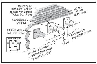
Figure 6. Exhaust and Combustion Air Pipe Clearances
