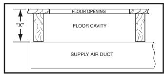
Figure 12. Floor Cavity
