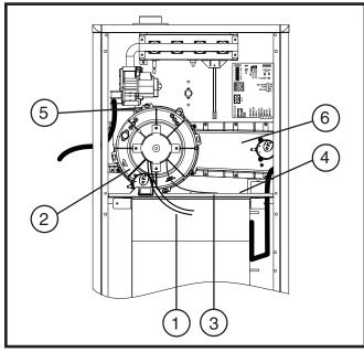
Figure 25. Inducer Assembly Rotation
