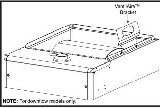
Figure 31. VentilAire™ Bracket
