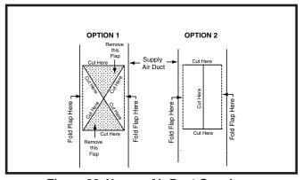
Figure 20. Narrow Air Duct Openings
