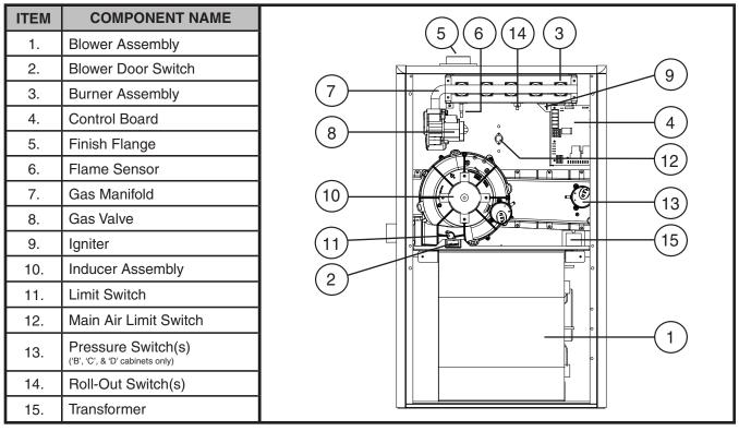
Figure 45. Upflow Gas Furnace Components
