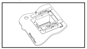
Figure 15. Duct Connector Side Plates
