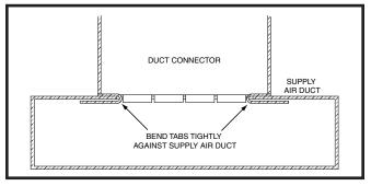
Figure 16. Duct Connector Tabs
