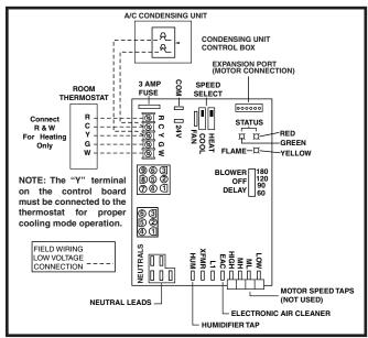
Figure 37. Low Voltage Field, Four-wire Heating / Cooling Applications
