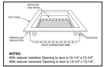
Figure 11. Duct Connector
