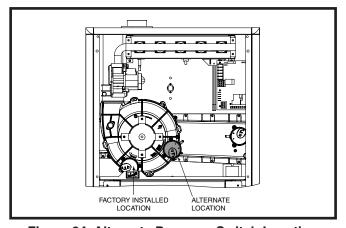
Figure 24. Alternate Pressure Switch Location
