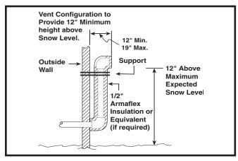
Figure 8. Alternate Horizontal Vent Installation
