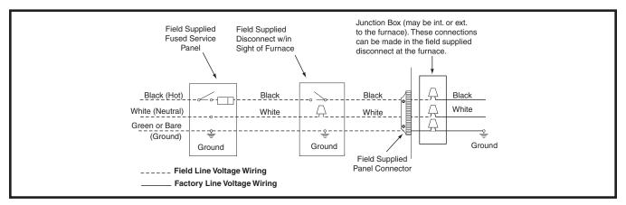
Figure 38. Line Voltage Field Wiring
