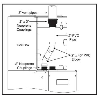
Figure 33. Alternate vent Pipe Installation
