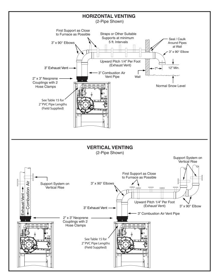
Figure 42. Horizontal and Vertical Venting
