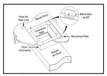
Figure 14. Duct Connector Installed
