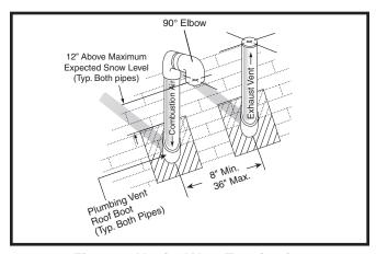
**Figure 9. Vertical Vent Termination**
