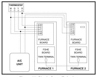
Figure 39. Single Stage Twinning
