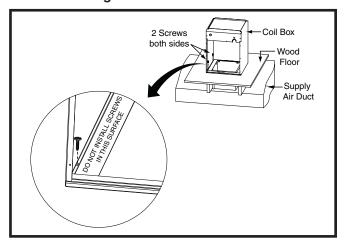
Figure 18. A/C Coil Box Installation
