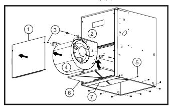
Figure 22. Bottom Panel Removal
