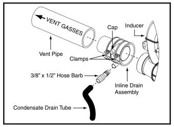
Figure 28. Inline Drain Assembly
