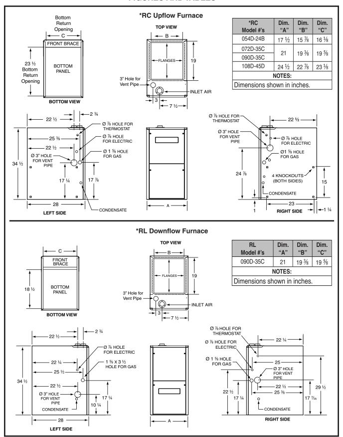
Figure 40. Furnace Dimensions
