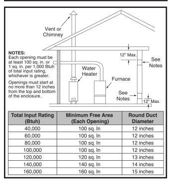
Figure 1. Combustion Air Drawn from Inside
