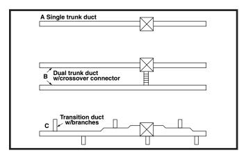
Figure 10. Typical Supply Duct System
