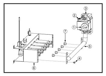
Figure 34. Burner and Manifold Assembly
