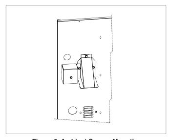
**Figure 6. Ambient Sensor Mounting**
