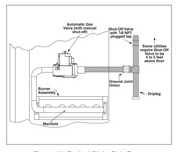
Figure 10. Typical Right Side Entry Gas Service Connection.
