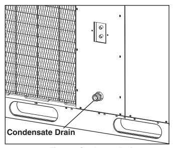
Figure 7. Condensate Drain
