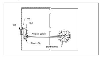
**Figure 5. Ambient Sensor Mounting**
