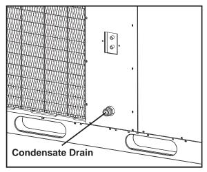
Figure 4. Condensate Drain
