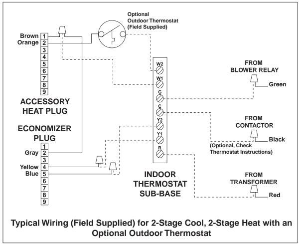
**Figure 8. Typical Air Conditioner Thermostat Connections**
