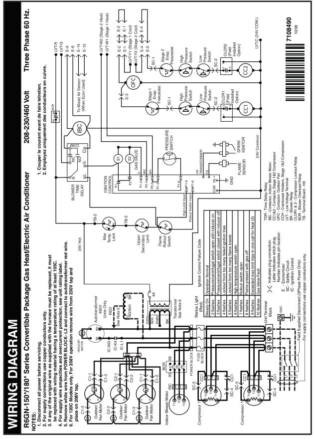
Figure 15. Ladder Diagram - 150/180 Series
