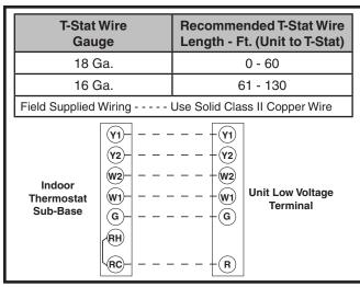
Figure 10. Typical 2 - Stage Heat/Cool Thermostat Connection
