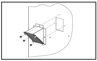
**Figure 2. Vent Cover Assembly**
