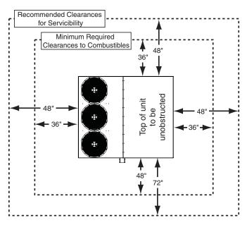
Figure 6. Unit Clearance Requirements
