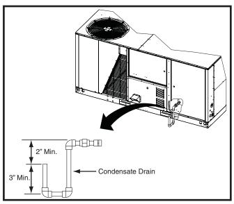
Figure 1. Condensate Drain
