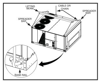
Figure 5. Rigging and Hoisting
