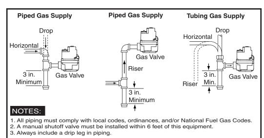
Figure 9. Typical Gas Service Connection.
