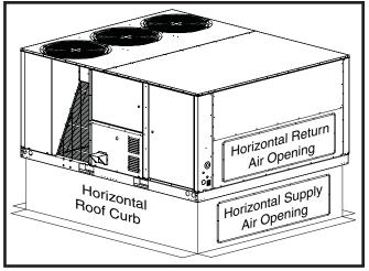
Figure 7. Horizontal Roof Curb
