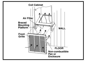
Figure 15. Over-the-Floor Return Air System
