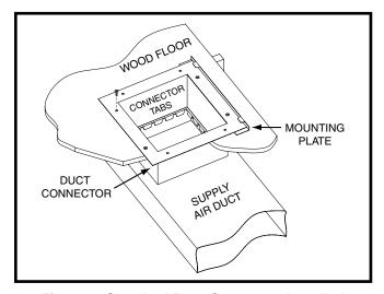
Figure 8. Standard Duct Connector Installed
