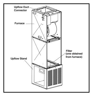
Figure 16. Over-the-Floor Return Air System with Upflow Stand
