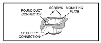
Figure 12. Round Duct Connector Installed
