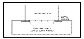
Figure 9. Duct Connector Tabs
