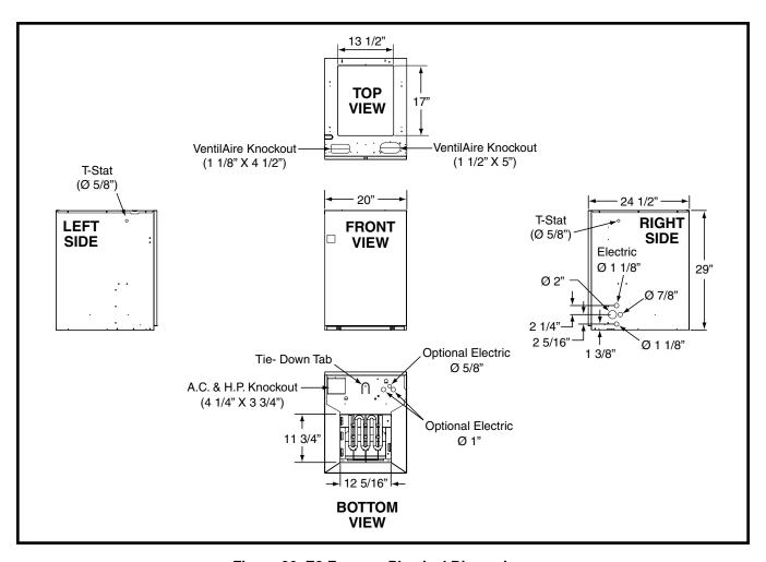
Figure 20. E3 Furnace Physical Dimensions
