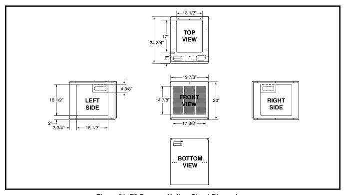
Figure 21. E3 Furnace Upflow Stand Dimensions
