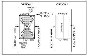
Figure 10. Narrow Air Duct Openings
