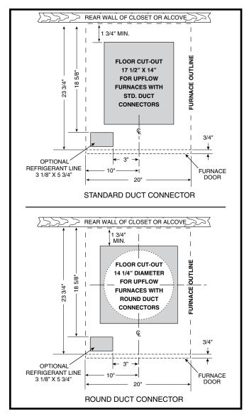
Figure 5. Cut-Out Dimensions for Upflow Furnaces
