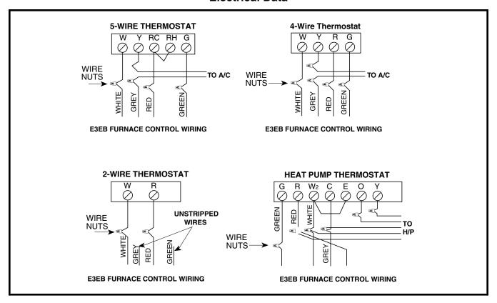
Figure 22. E3EB Thermostat Connection
