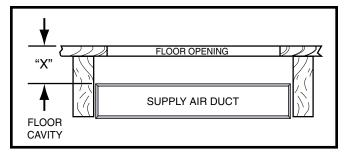
Figure 7. Floor Cavity
