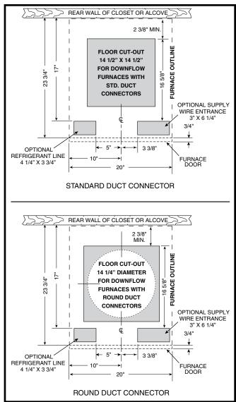
Figure 6. Cut-Out Dimensions for Downflow Furnaces
