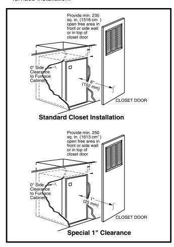
Figure 14. Closet Installation
