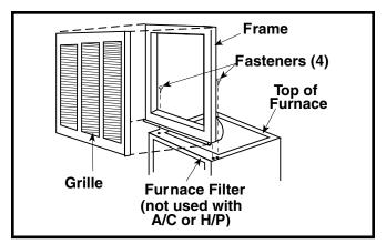
Figure 2. Grille Support Frame & Grille Assembly
