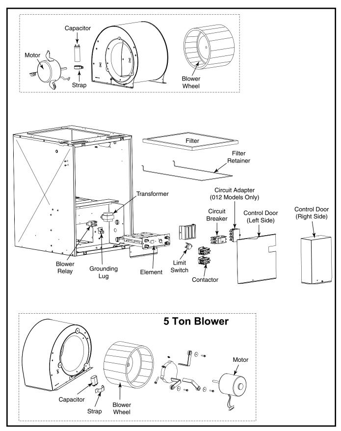
Figure 19. E3 Furnace Components
