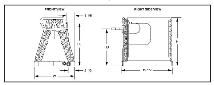
Figure 1. Coil Dimensions
