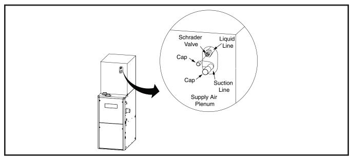
Figure 2. Suction and Liquid Line Locations
