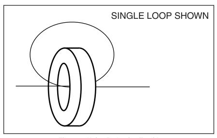
Figure 3. Noise Reduction Toroid
