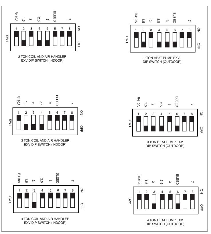
Figure 8. EXV Board DIP Switch Settings
