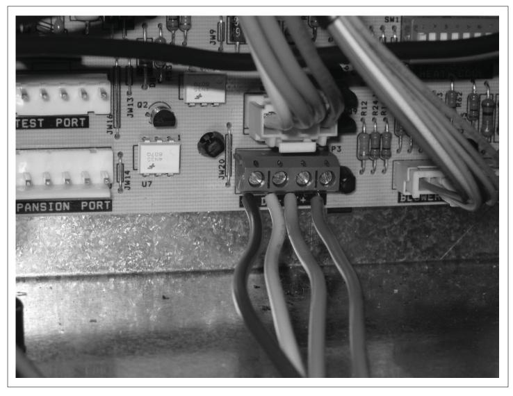
Figure 23. Control Wire Connections to Outdoor iQ Unit from Motor control Board
