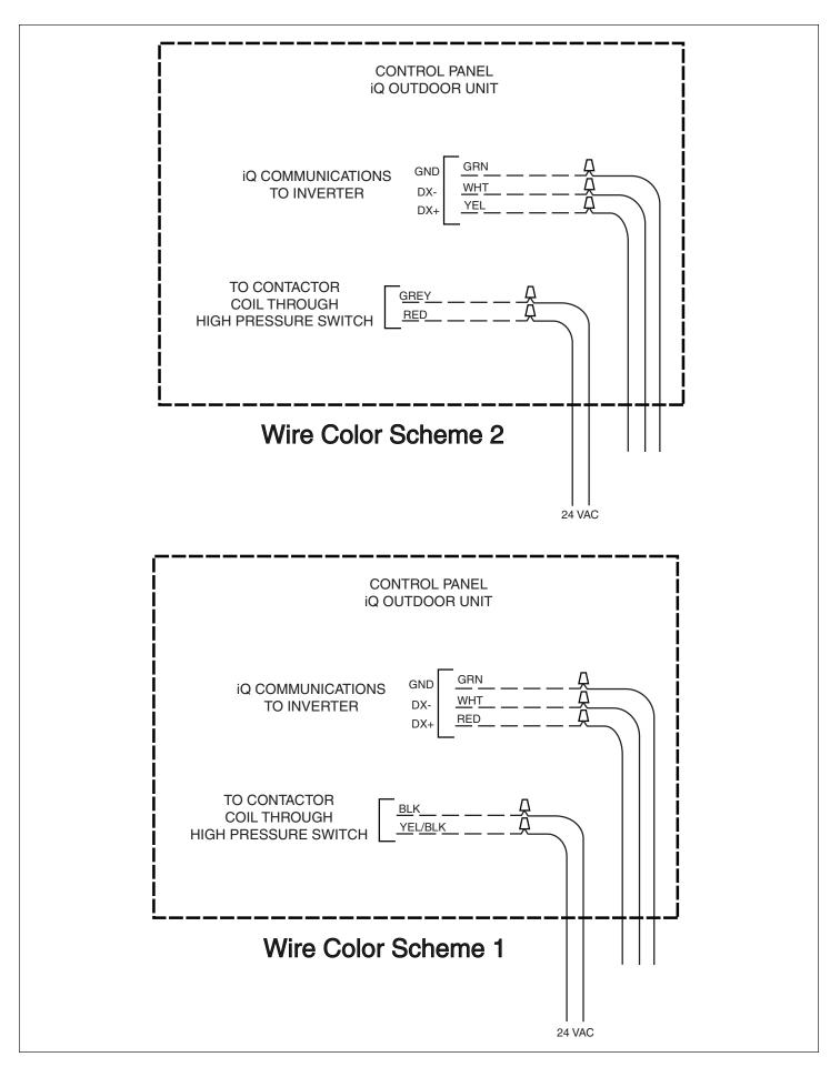
Figure 4A. Control Wiring Connections, iQ Air Conditioning Outdoor Unit
