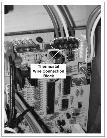
Figure 21. Modulating Gas Furnace Board Thermostat Connection
