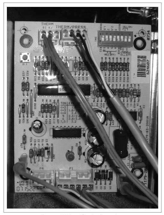
Figure 11. EXV Board Showing Connections
