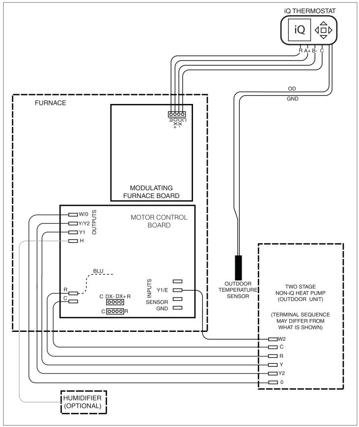
Figure 27. Control Wire Connections, G7 Modulating Gas Furnace with non-iQ
