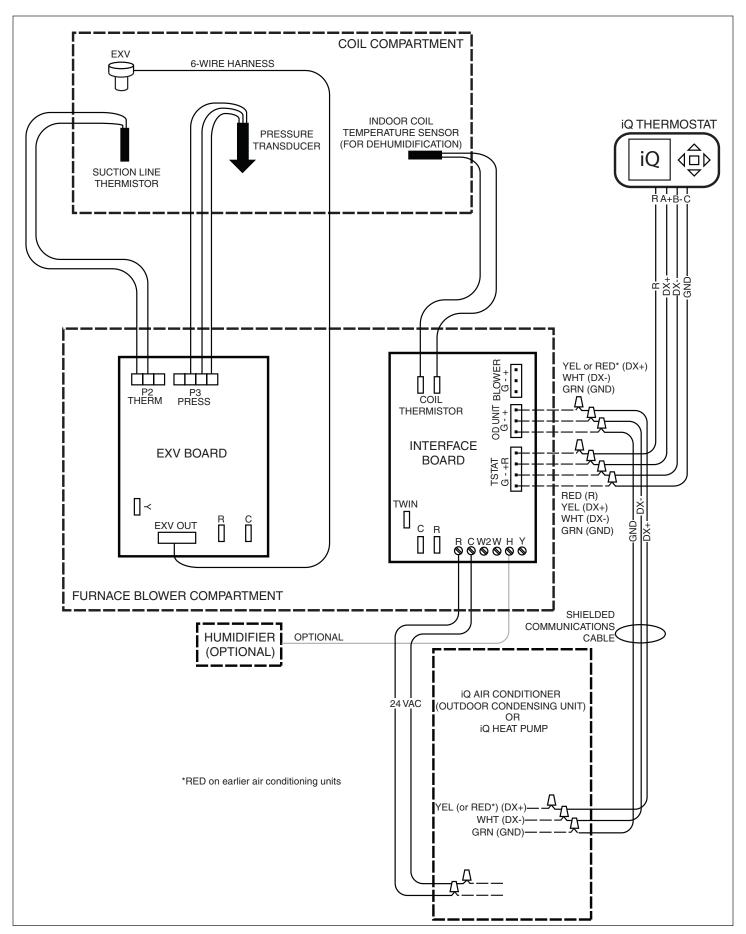
Figure 12. Control Wiring Between Interface Board, iQ Thermostat, and Outdoor Unit (G6 Gas Furnaces and B5VM/B4VM Air Handlers)
