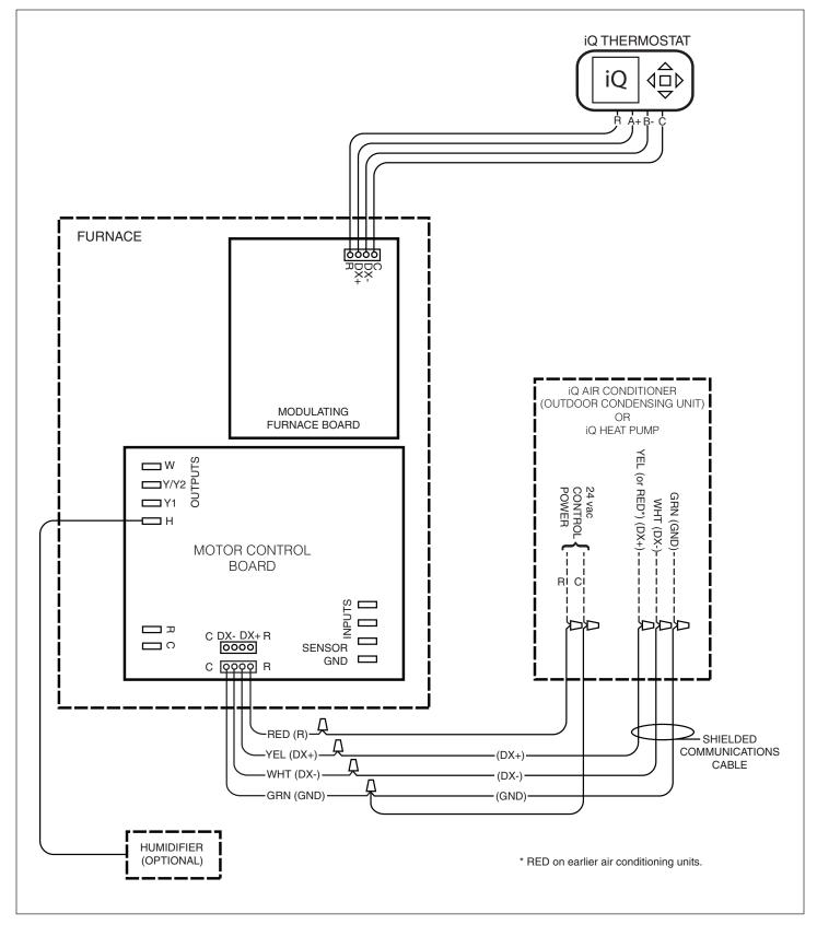
Figure 22. Control Wire Connections, G7 Modulating Gas Furnace
