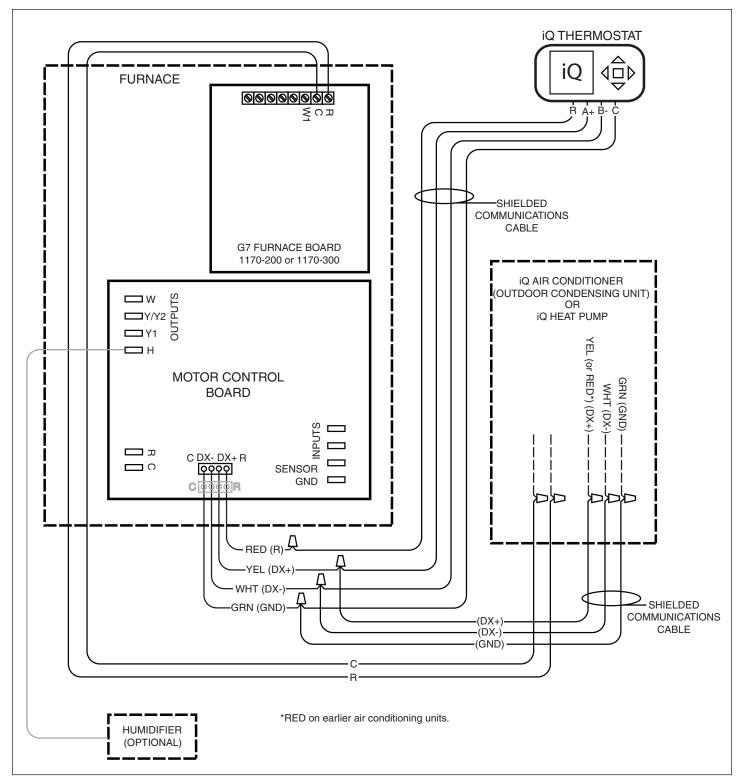
Figure 17. Control Wire Connections, G7 Single and Two Stage Furnaces
