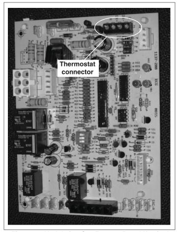
Figure 20. Modulating Gas Furnace Board Unwired
