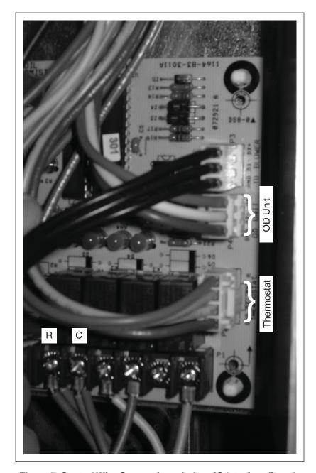
Figure 7. Control Wire Connections. Indoor iQ Interface Board.
