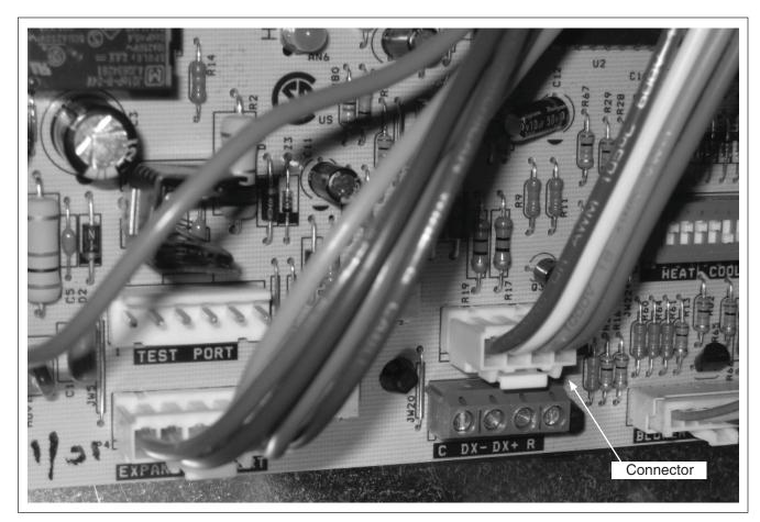
Figure 16. Four-wire connector on Motor Control Board
