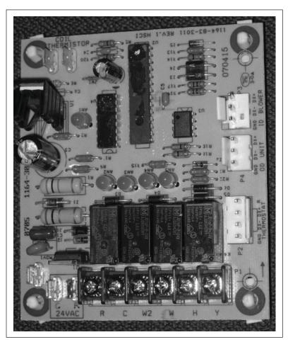
Figure 6. Indoor iQ Interface Board Unwired
