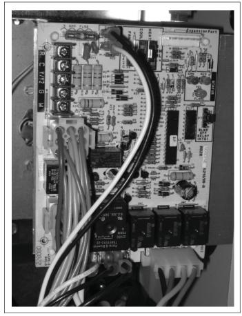
Figure 18. Single Stage G7 Furnace Board
