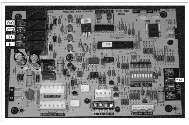
Figure 13. Blower Motor Control Board Unwired
