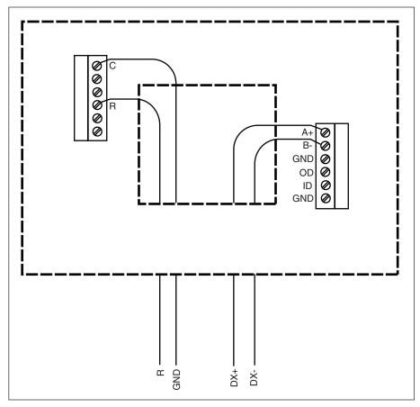
Figure 1A. iQ Controller/Thermostat Back Plate Wiring
