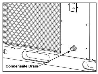
Figure 4. Condensate Drain.
