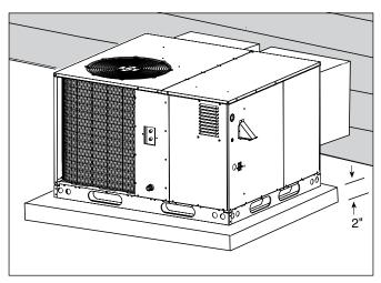
Figure 5. Ground Level Installation.
