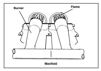
Figure 11. Burner Inspection
