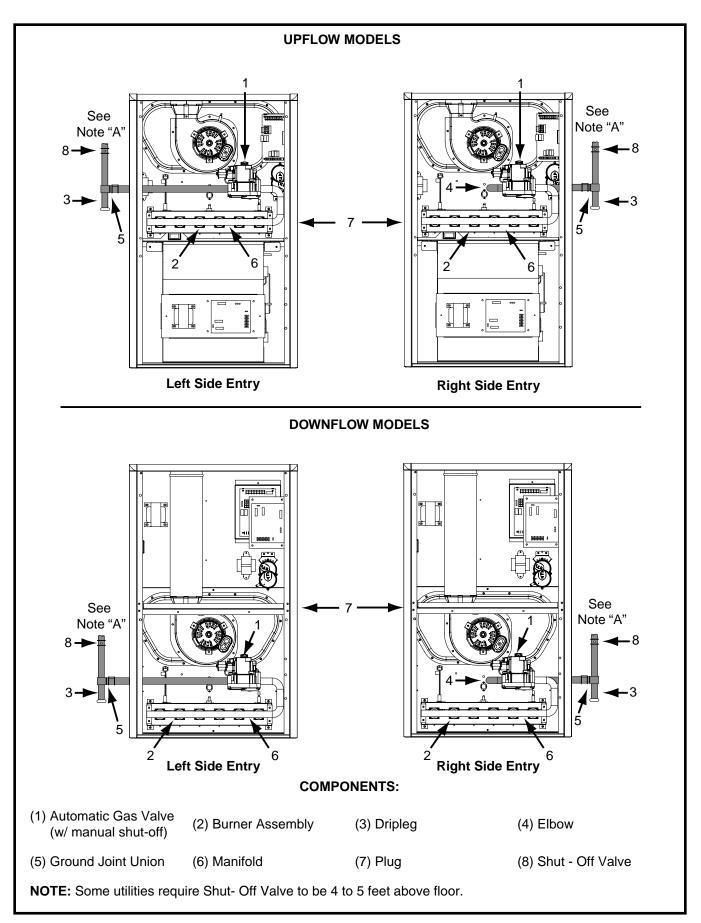
Figure 13. Typical Gas Connections
