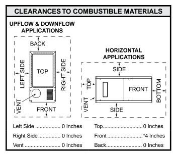
$^{\dagger}\text{Allow}$  24 in. minimum clearance for servicing. Recommended clearance is 36 in.
