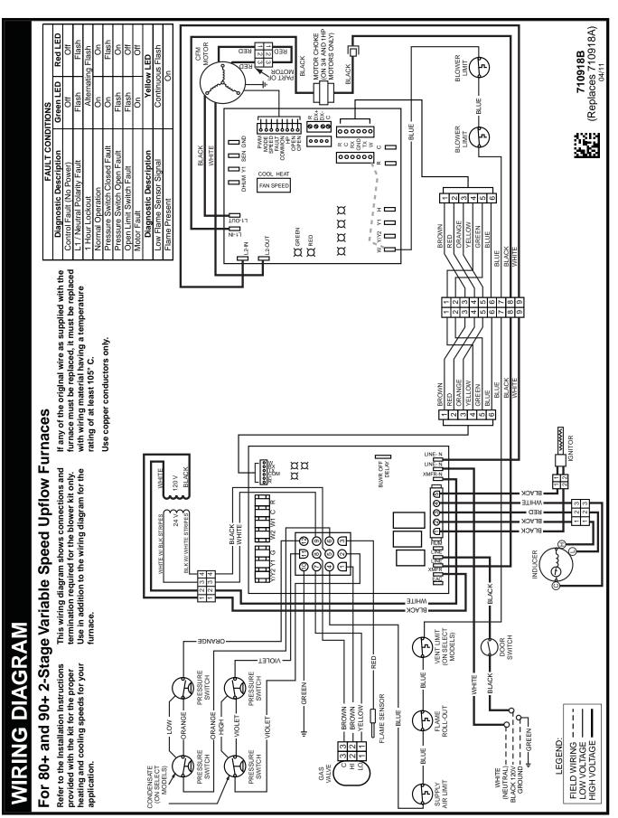
Figure 27. Wiring Diagram for Two-Stage, Variable Speed Upflow Furnaces
