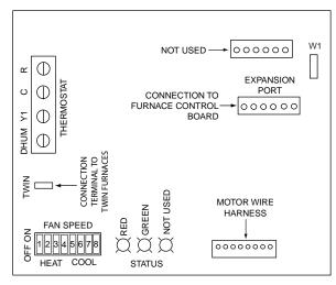
Figure 22. Two-Stage Fixed Speed Motor Control Board
