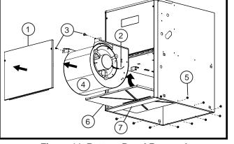
Figure 11. Bottom Panel Removal
