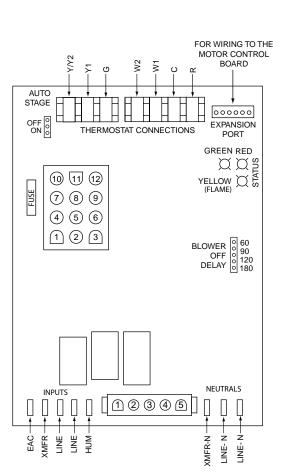
Figure 24. Two-Stage Furnace Control Board
