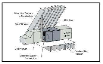
Figure 7. \*TA Horizontally Installed on a Platform
