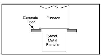
Figure 9. Furnace on a Concrete Slab
