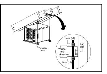
Figure 8. \*TA Horizontally Suspended in Attic
