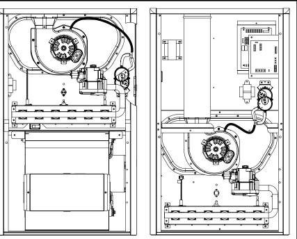
Figure 10. Pressure Switch Tubing for \*TA & \*TK Furnaces
