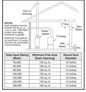
Figure 1. Combustion Air Drawn from Inside
