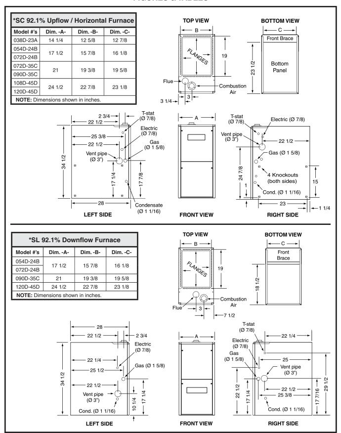
Figure 31. Furnace Dimensions
