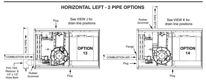
Figure 36. Horizontal Options - 2-pipe Furnaces
