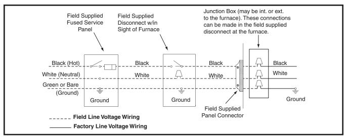
Figure 27. Line Voltage Field Wiring
