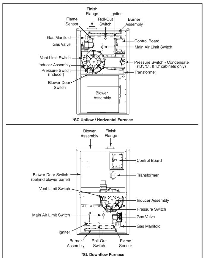
Figure 38. Furnace Components
