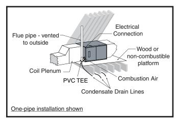
Figure 12. \*SC Horizontal installation on a Platform
