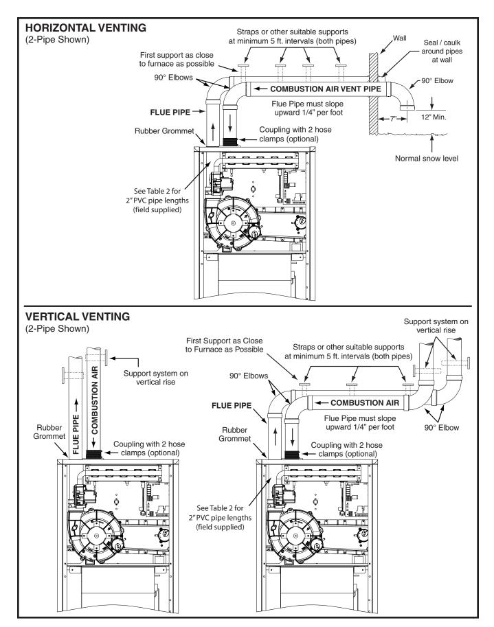
Figure 33. Horizontal & Vertical Venting
