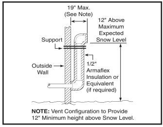
Figure 8. Alternate Horizontal Vent Installation
