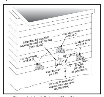
Figure 6. Inlet & Exhaust Pipe Clearances
