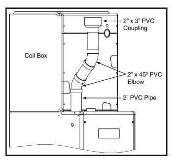
Figure 23. Optional PVC Pipe Installation
