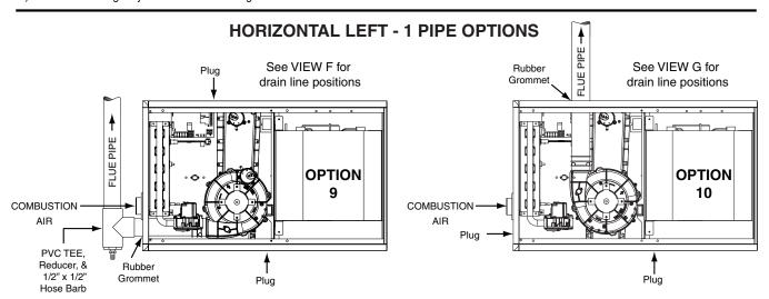
Figure 35. Horizontal Options - 1 Pipe Furnaces
