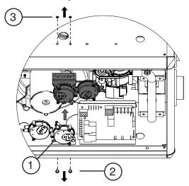
Figure 14. SC038-23A Pressure Switch
