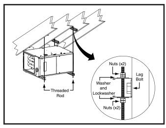
Figure 13. \*SC Horizontally Suspended in Attic
