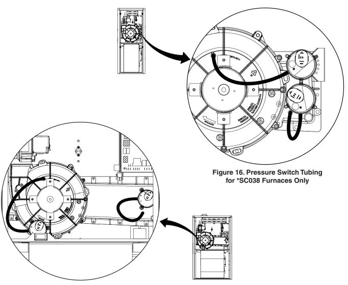
Figure 17. Pressure Switch Tubing for Upflow Furnaces (Models: \*SC054, \*SC072, \*SC090, \*SC108, & \*SC120)
