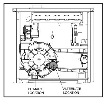
Figure 19. Alternate Pressure Switch Location
