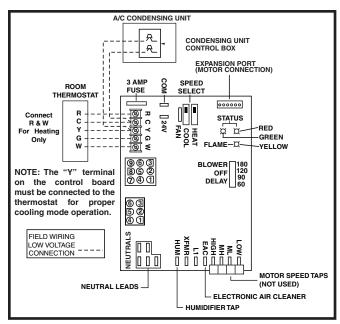
Figure 28. Low Voltage Field, Four-wire Heating/Cooling Applications
