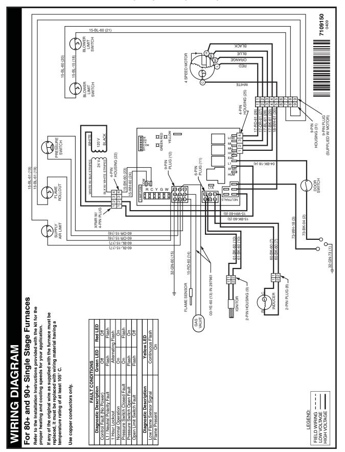
Figure 32. Wiring Diagram for Upflow & Downflow Furnaces
