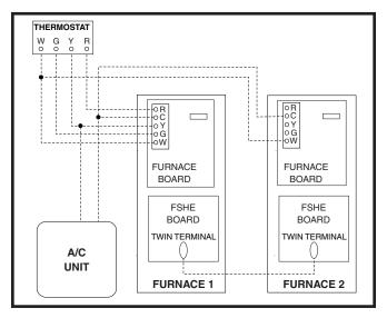
Figure 29. Single Stage Twinning
