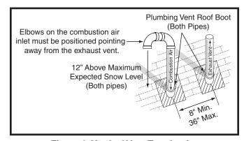
**Figure 9. Vertical Vent Termination**
