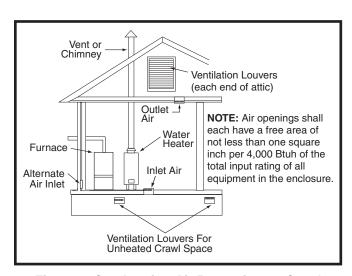
Figure 2. Combustion Air Drawn from a Crawl Space or Vented Attic
