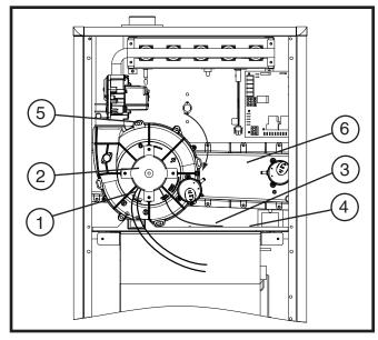
Figure 15. Inducer Assembly Rotation
