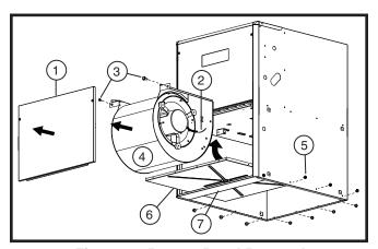
Figure 24. Bottom Panel Removal
