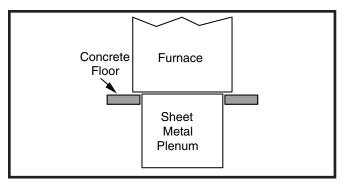
Figure 11. Furnace on a Concrete Slab
