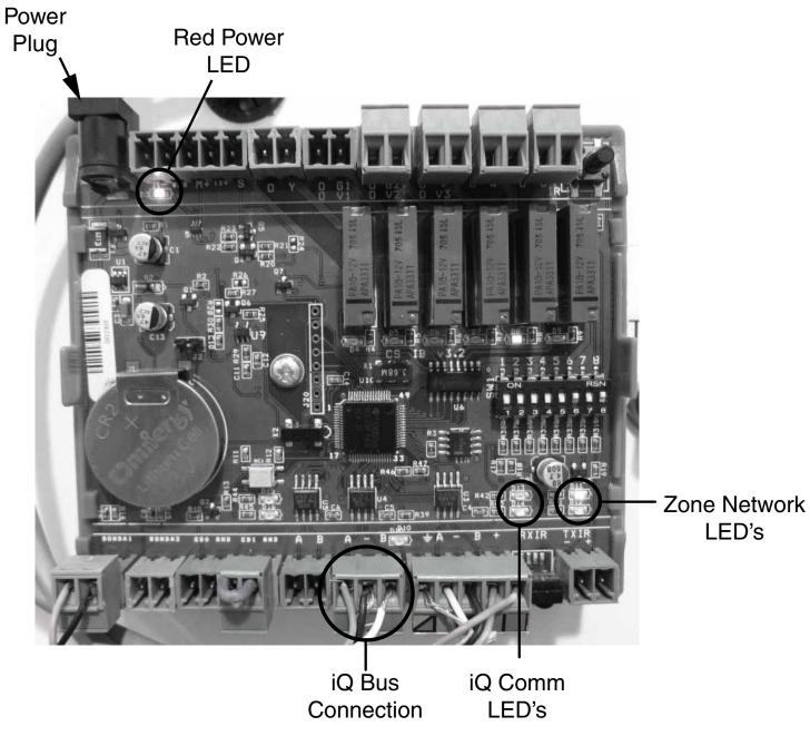
Figure 12. iQ Control Board LED locations
