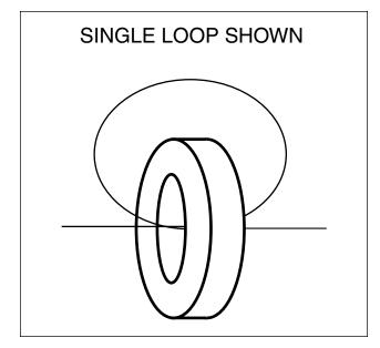
Figure 7. Wire Looping Through a Toroidial Choke
