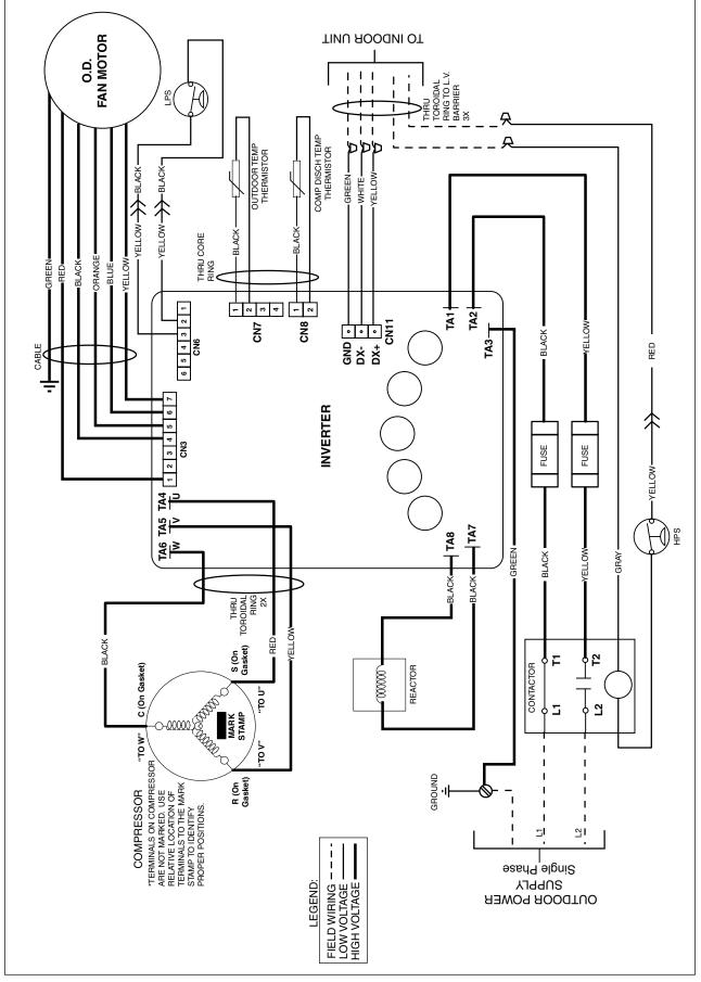
Figure 4. iQ Drive Air Conditioning Wiring Diagram
