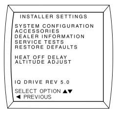
Other than in the splash screen displayed when power is first applied to the controller, this is the only screen which displays the controller software version number.
