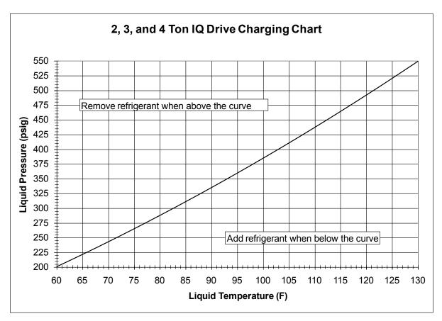
Figure 9. Charging Chart for iQ Drive Air Conditioning
