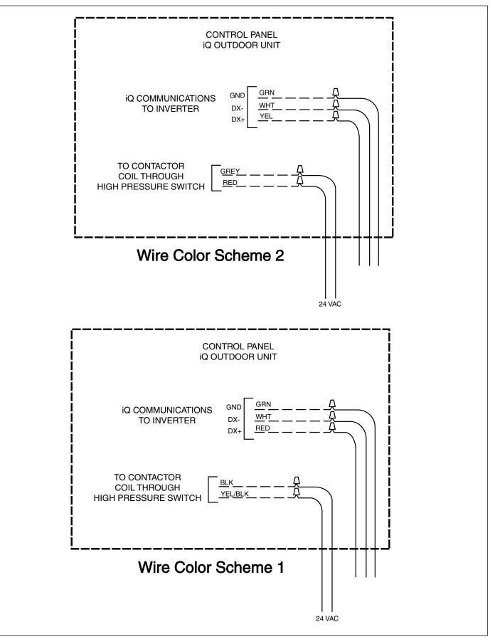
Figure 6. iQ Drive Air Conditioning Control Wiring Connections
