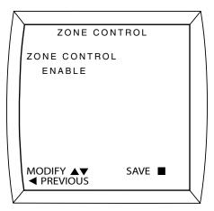
To restore zone control (when the zoning system components are functioning properly), follow the above sequence, but in step 7 change DISABLE to ENABLE.
