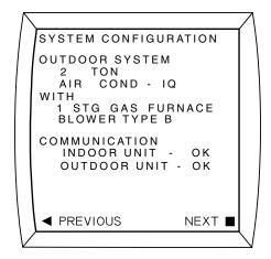
The words under OUTDOOR SYSTEM and WITH describe the system components as automatically detected by the controller. Both entries under COMMUNICATION should show "OK". If "CHECK" appears, it is an indication that either communication wiring is incomplete or incorrect, or the outdoor unit is not powered up. Proceed through subsequent screens by using either the  $\blacktriangleright$  or  $\blacksquare$  key (indicated by "NEXT").
