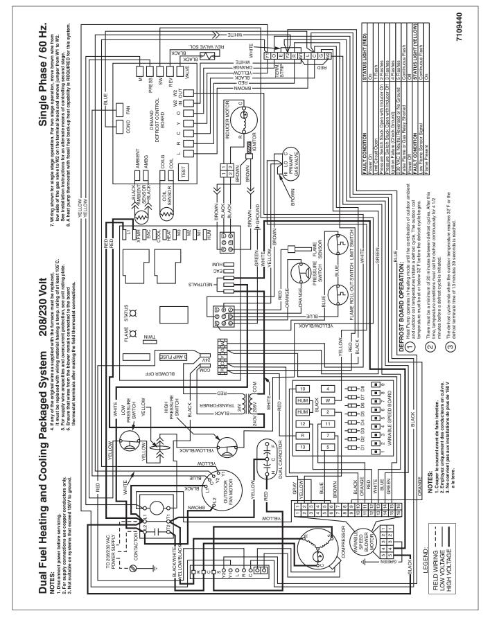
Figure 13c. Two Stage Cool, Two Stage Heat (Heat Pump) High Fire Only-Gas Heating "With Optional Comfort Alert" (3 & 4 Ton)
