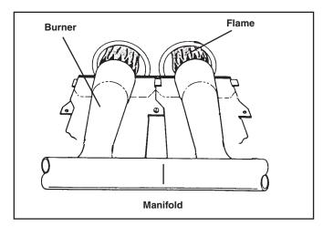
Figure 11. Burner Inspection
