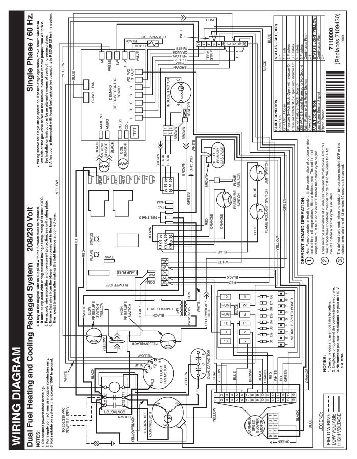
Figure 13b. Two Stage Cool, Two Stage Heat (Heat Pump) High Fire Only-Gas Heating (3 & 4 Ton)
