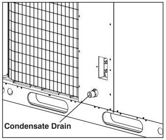
Figure 7. Condensate Drain
