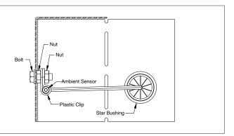
Figure 5. Ambient Sensor Mounting
