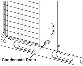
Figure 4. Condensate Drain.
