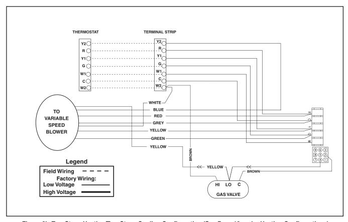
Figure 8b. Two Stage Heating/Two Stage Cooling Configuration (See Page 12 under Heating Configurations)
