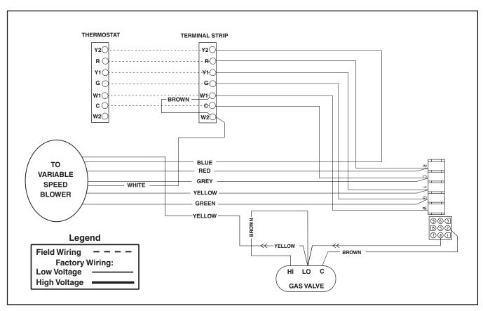
Figure 8a. High Fire Only Configuration (As shipped from the factory)
