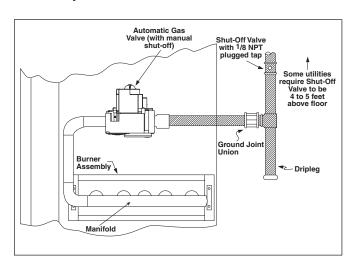
Figure 7. Typical Right Side Entry Gas Service Connection.
