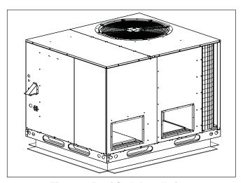
Figure 6. Roof Curb Installation.
