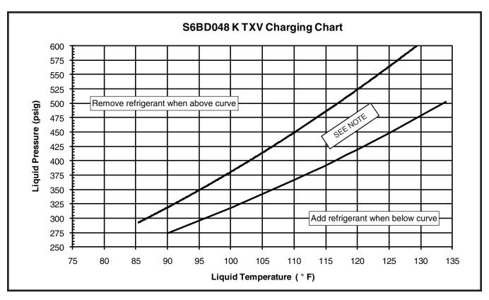
Figure 11. Charging Chart for 4 Ton Units
