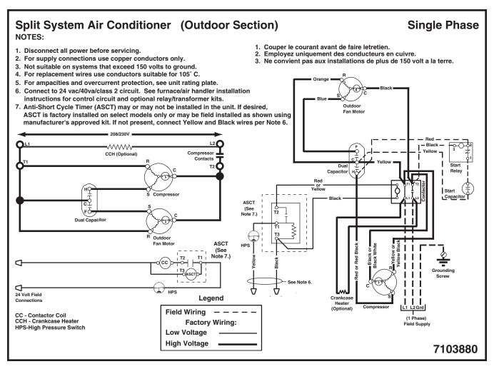
Figure 6. JS6BD Wiring Diagram (3.5 & 5 Ton Units)
