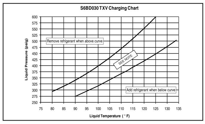
Figure 8. Charging Chart for 2.5 Ton Units
