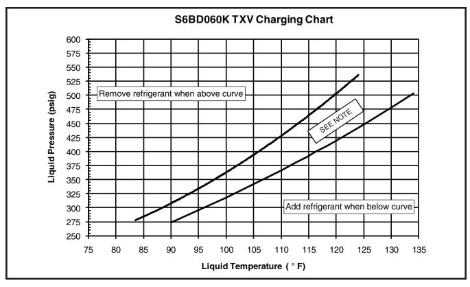
Figure 12. Charging Chart for 5 Ton Units
