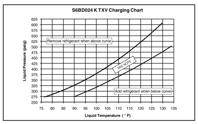
Figure 7. Charging Chart for 2 Ton Units
