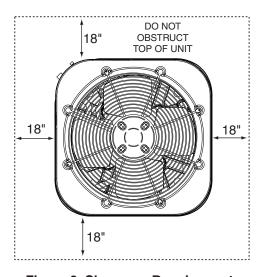
Figure 2. Clearance Requirements
