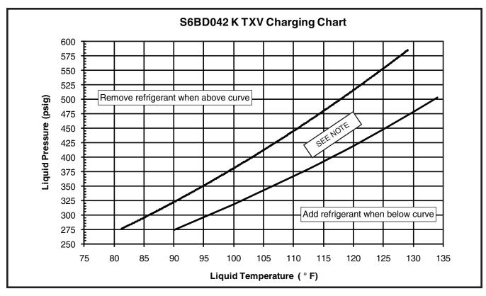
Figure 10. Charging Chart for 3.5 Ton Units
