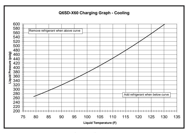
Figure 13. Charging Chart for 5 Ton Units
