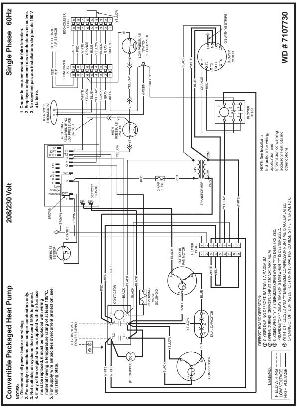
Figure 10: Wiring Diagram
