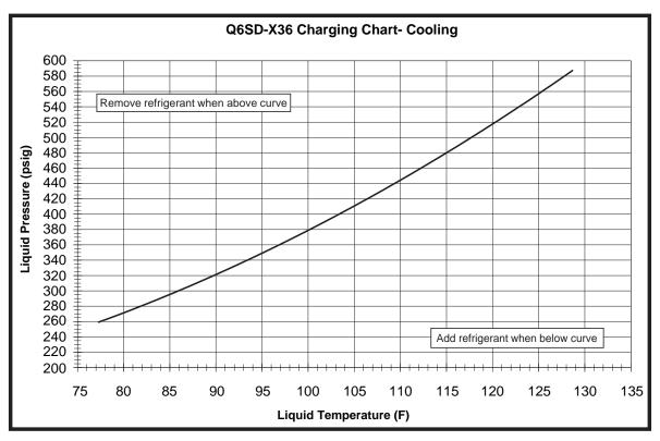
Figure 10. Charging Chart for 3 Ton Units
