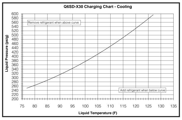
Figure 9. Charging Chart for 2.5 Ton Units
