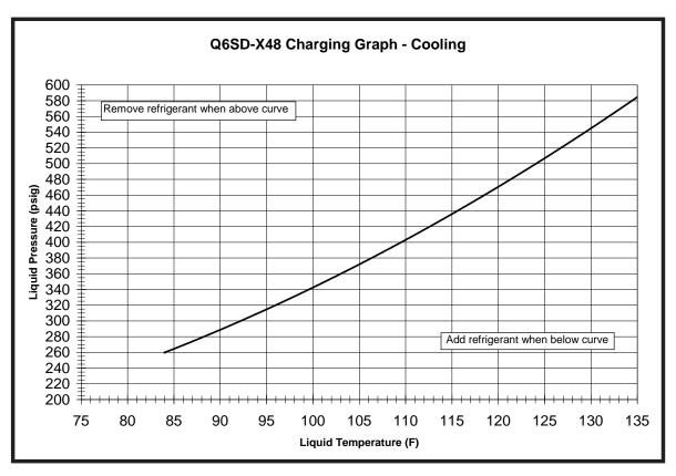
Figure 12. Charging Chart for 4 Ton Units
