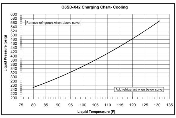
Figure 11. Charging Chart for 3.5 Ton Units
