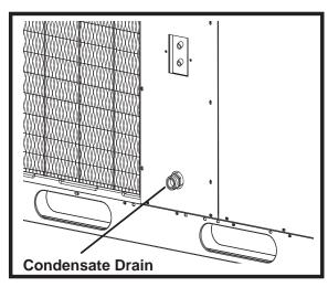
Figure 4. Condensate Drain
