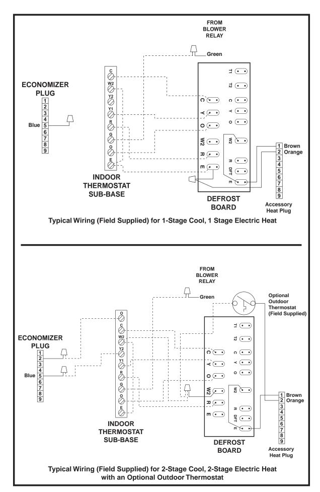
Figure 7. Typical Heat Pump Thermostat Connections
