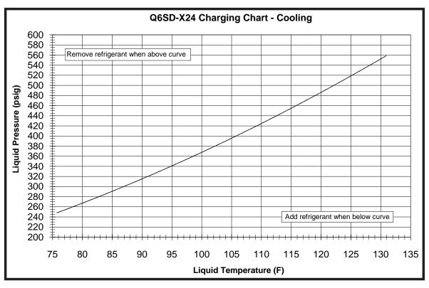
Figure 8. Charging Chart for 2 Ton Units
