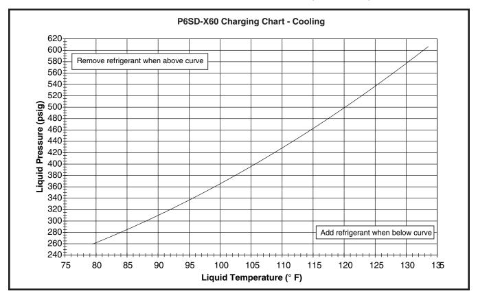
Figure 20. Charging Chart for 2 Ton Units
