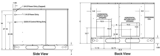
Figure 9. P6SD Air Conditioner Dimensions
