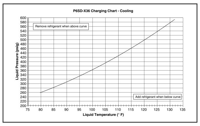
Figure 18. Charging Chart for 3 Ton Units
