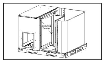
Figure 5. Internal Filter Rack Location
