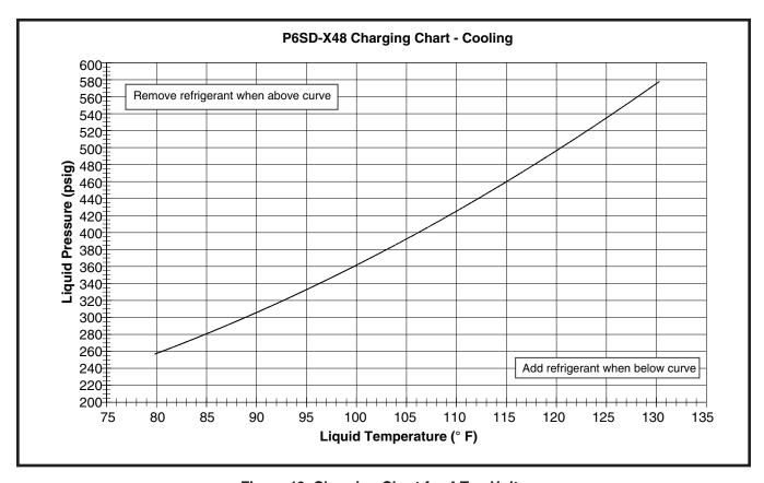
Figure 19. Charging Chart for 4 Ton Units
