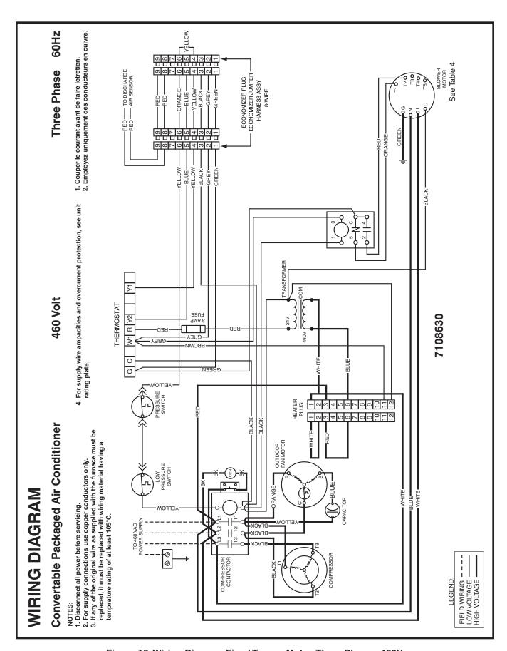
Figure 16. Wiring Diagram-Fixed Torque Motor, Three Phase - 460V
