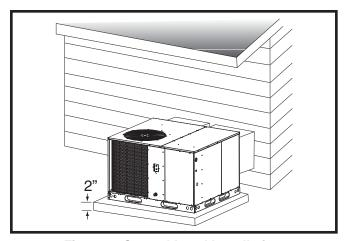
Figure 3. Ground Level Installation
