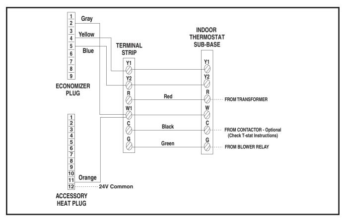
Figure 11. Typical Air Conditioner Thermostat Connections - 460V
