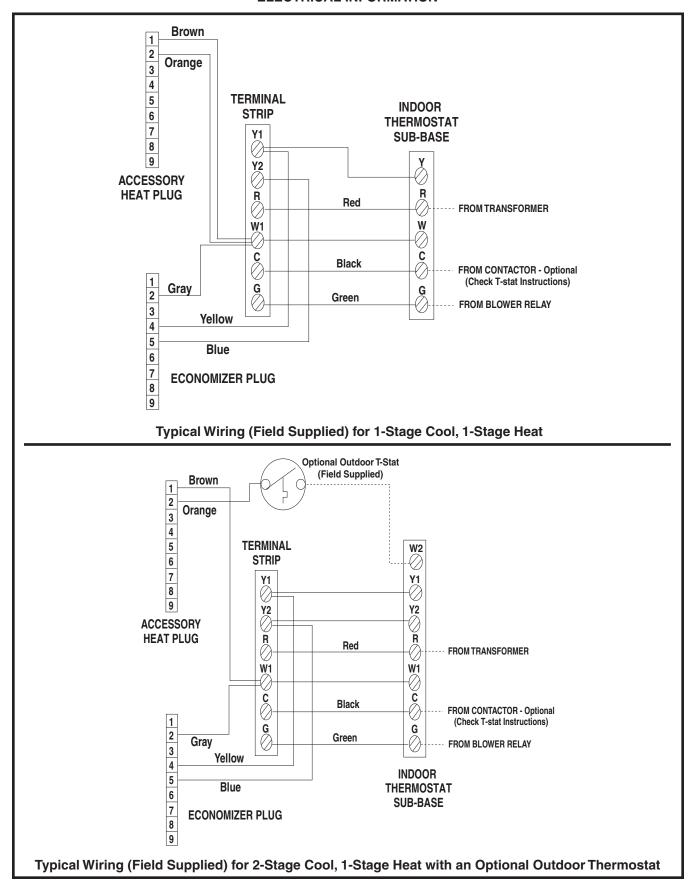
Figure 10. Typical Air Conditioner Thermostat Connections - 208/230V
