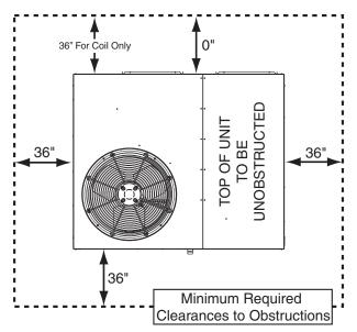
Figure 2. Clearance Requirements
