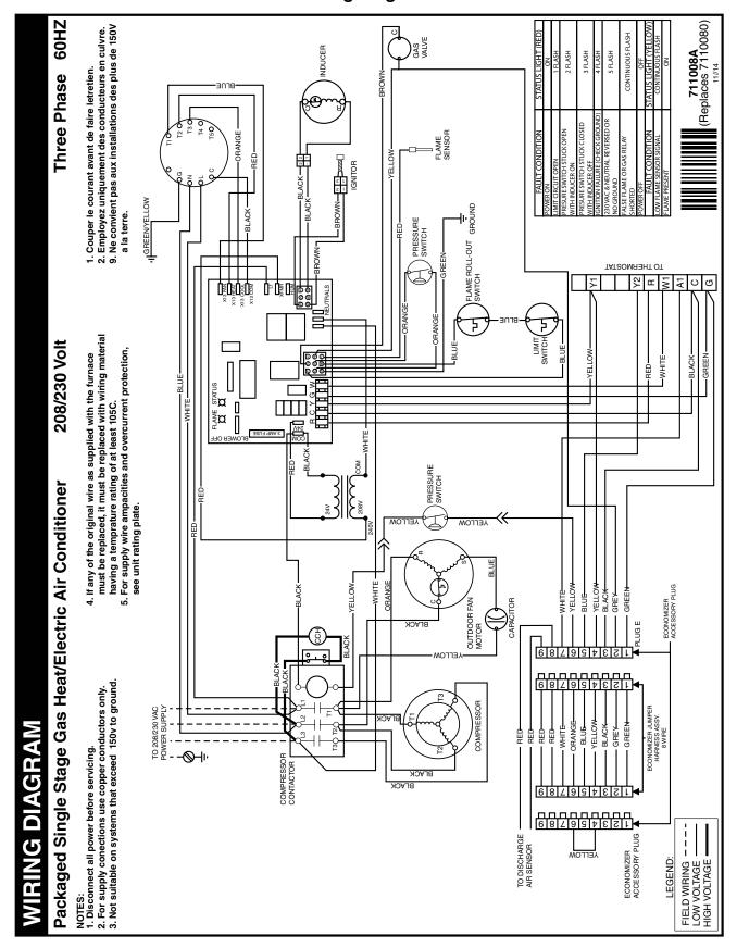
Figure 12. Wiring Diagram for 208/230V / 3 Phase / 60 Hz Unit
