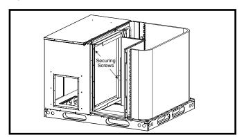
Figure 7. Internal Filter Rack Location
