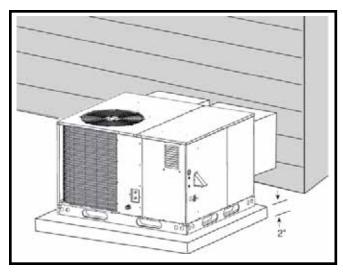
Figure 4. Ground Level Installation
