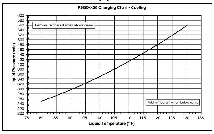
Figure 14. Charging Chart for 3 Ton Units
