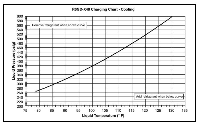
Figure 15. Charging Chart for 4 Ton Units
