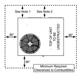
Figure 2. Clearance Requirements
