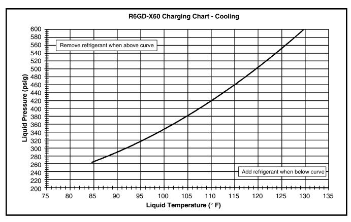
Figure 16. Charging Chart for 5 Ton Units
