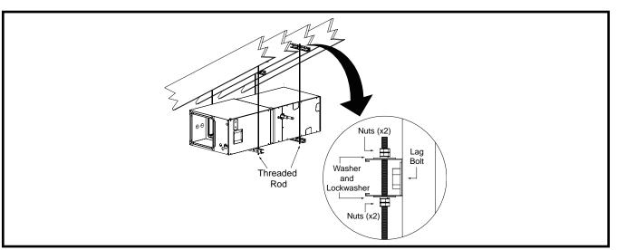
Figure 5. Unit Horizontally Suspended
