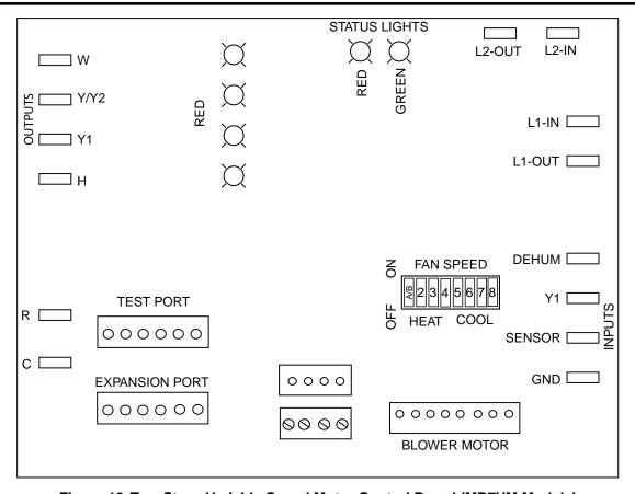
Figure 13. Two-Stage Variable Speed Motor Control Board (MB7VM Models)
