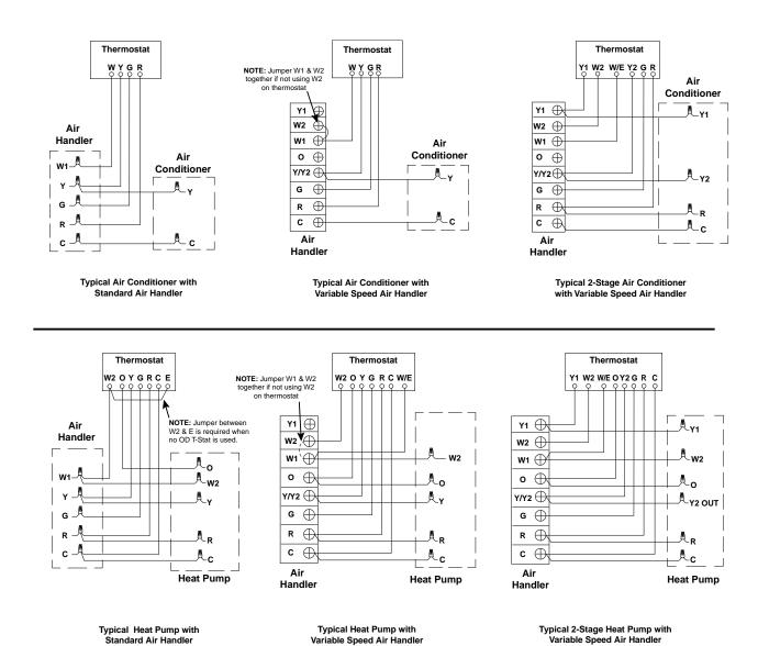
**Figure 9. Typical Thermostat Connections**
