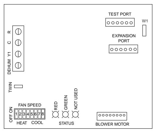
Figure 12. Fixed Speed Motor Control Board (MB7EM Models)
