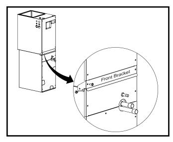
Figure 3. Front Bracket Installation - (Upflow Only)
