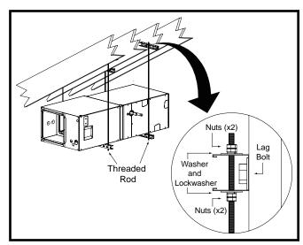
Figure 5. Unit Horizontally Suspended
