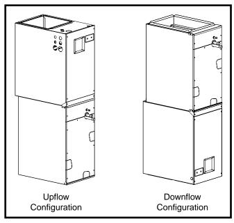
Figure 1. Upflow & Downflow Installation
