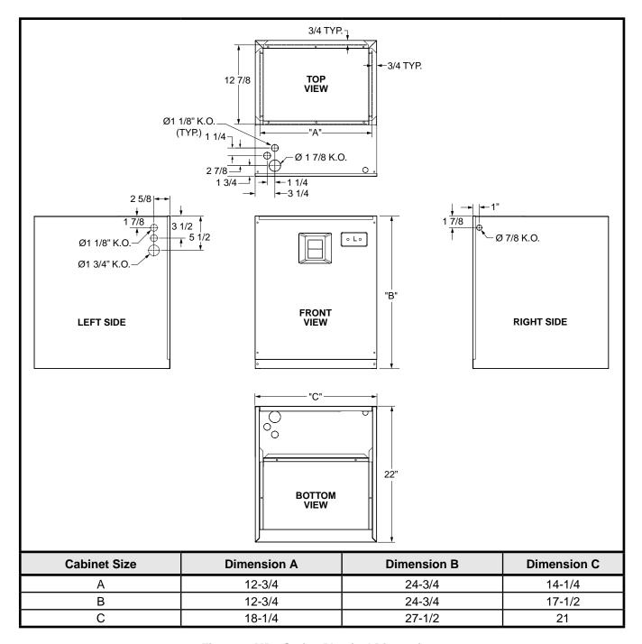
Figure 7. MB7 Series Physical Dimensions
