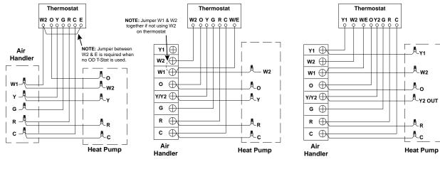
**Figure 9. Typical Thermostat Connections**
