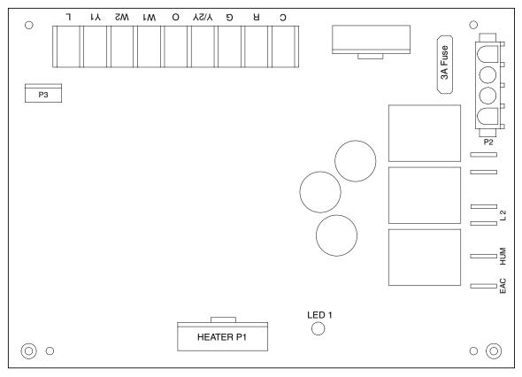
Figure 11. Two - Stage Control Board (MB7EM & MB7VM Models)
