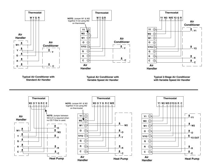
**Figure 9. Typical Thermostat Connections**
