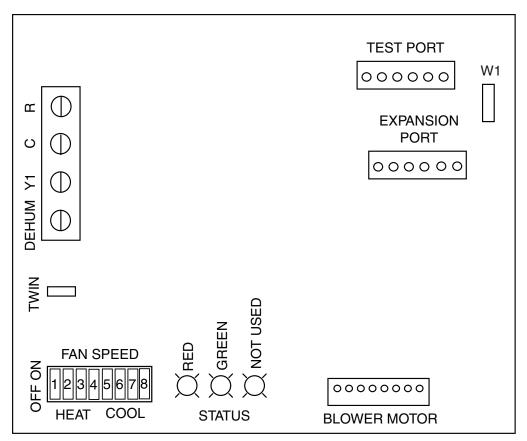
Figure 12. Fixed Speed Motor Control Board (MB7EM Models)
