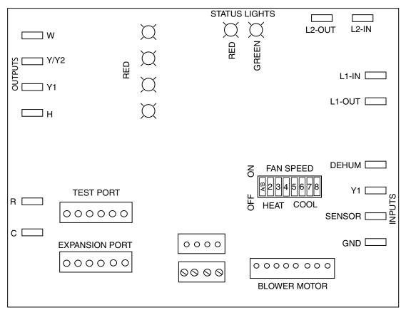
Figure 13. Variable Speed Motor Control Board (MB7VM Models)
