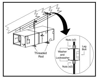
Figure 5. Unit Horizontally Suspended
