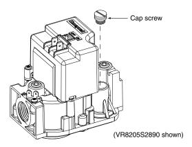
Figure 2. Cap Screw Removal
