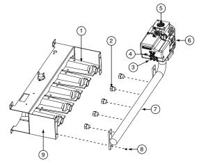
Figure 1. Burner & Manifold Assembly
