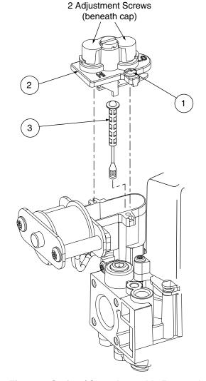
Figure 4. Spring / Stem Assembly Removal
