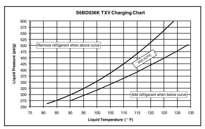
Figure 9. Charging Chart for 3 Ton Units
