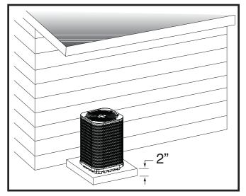
Figure 3. Ground Level Installation
