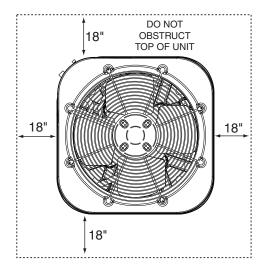
Figure 2. Clearance Requirements
