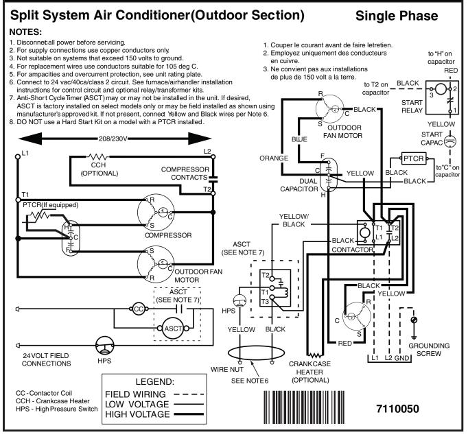
Figure 4. NS6BD Wiring Diagram (2 - 2.5 Ton Units)
