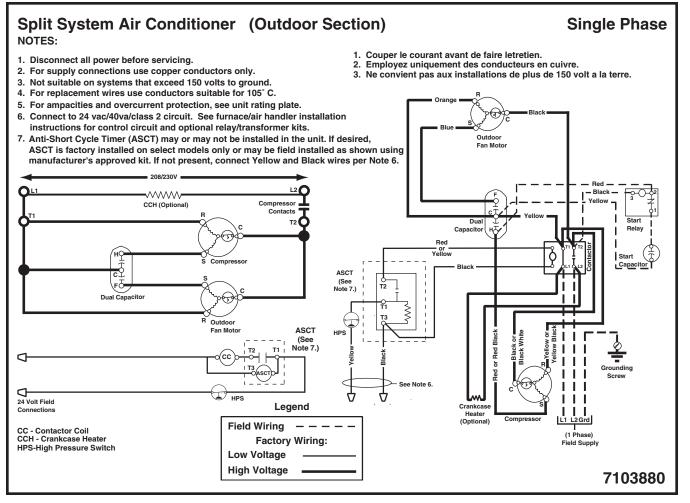
Figure 6. NS6BD Wiring Diagram (3.5 - 5 Ton Units)
