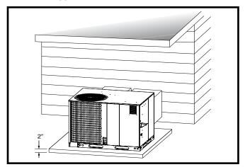
Figure 3. Ground Level Installation
