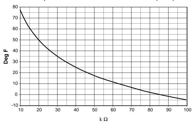
**Figure 23. Temperature Sensor Resistance Charts**
