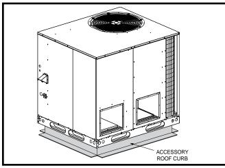
Figure 4. Roof Top Installation
