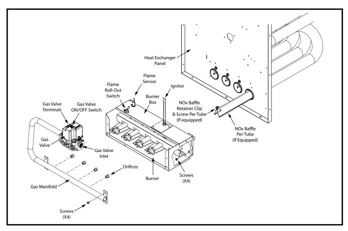
Figure 8. Burner & Manifold Assembly
