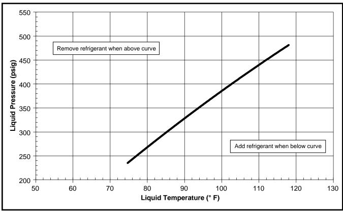
Figure 22. Charging Chart for 5 Ton Units
