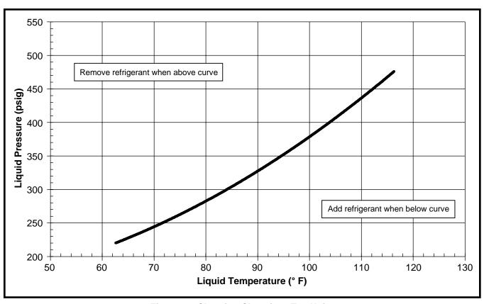
Figure 19. Charging Chart for 2 Ton Units
