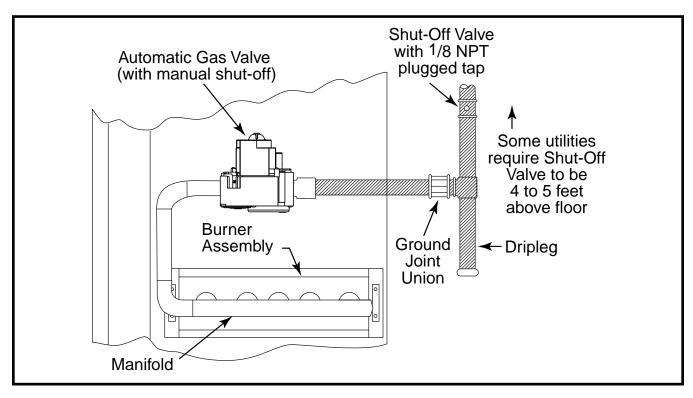
Figure 7. Typical Gas Hookup - Right Side Entry
