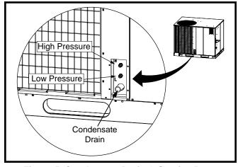
Figure 5. Condensate Drain & Service Ports
