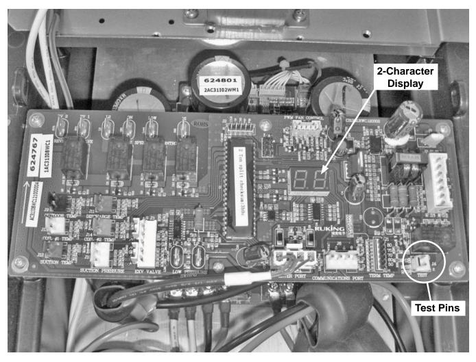
Figure 14. Interface Board in Control Panel
