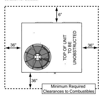
Figure 1. Clearance Requirements
