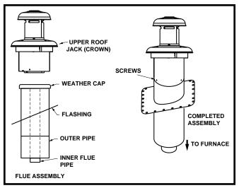
Figure 23. Roof Jack Crown
