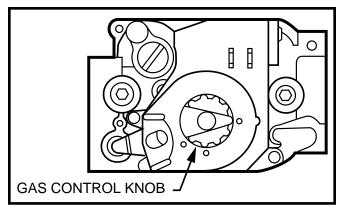
Figure 30. Direct Ignition Gas Valve - Honeywell
