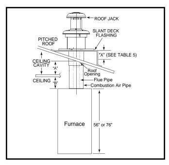
Figure 16. Ceiling Cavity Depth
