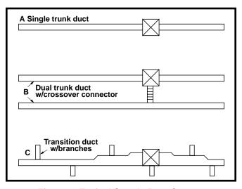
Figure 5. Typical Supply Duct System
