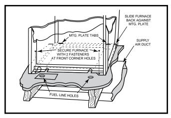
Figure 15. "A" Cabinet Furnace on Coil Cabinet
