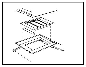
Figure 35. Damper without Coil Cavity
