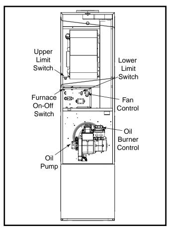
Figure 33. Furnace Controls - Oil Furnace
