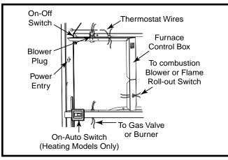
Figure 24. Control Panel (All Models)
