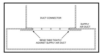
Figure 10. Duct Connector Tabs
