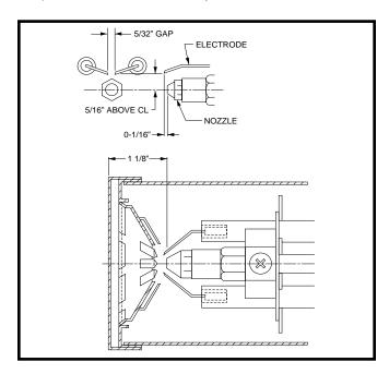
Figure 32. Oil Gun electrode Position
