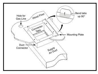
Figure 8. Standard Duct Connector Installed
