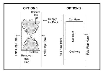
Figure 11. Narrow Air Duct Openings
