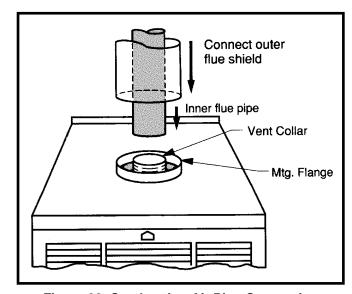
Figure 22. Combustion Air Pipe Connection
