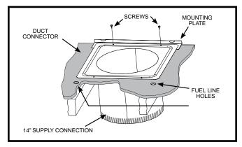
Figure 13. Round Duct Connector Installed
