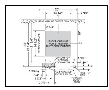
Figure 6. Cut-Out Dimensions for Standard Duct Connectors
