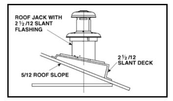
Figure 18. Example of 2½ / 12 Slant Jack with Flashing
