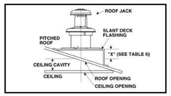
Figure 17. Example of Flat Jack with Flashing
