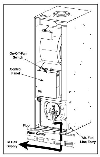
Figure 26. Typical Gas Piping
