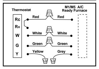
Figure 25. Thermostat Wiring For A/C Ready Models
