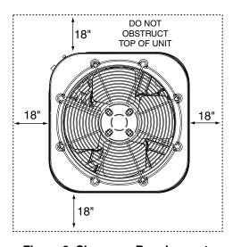
Figure 2. Clearance Requirements
