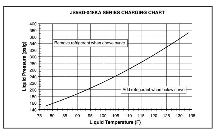
Figure 10. Charging Chart for 4 Ton Units
