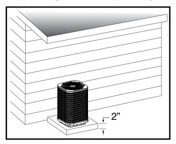
Figure 3. Ground Level Installation
