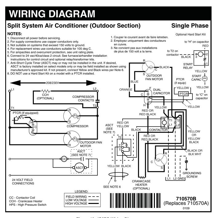
Figure 12. JS5BD Wiring Diagram
