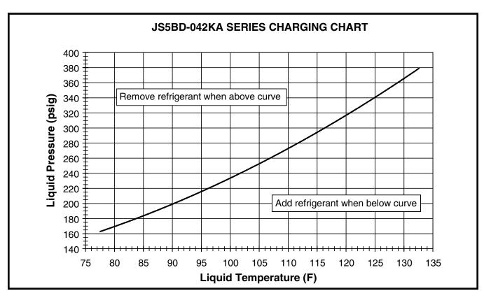
Figure 9. Charging Chart for 3.5 Ton Units
