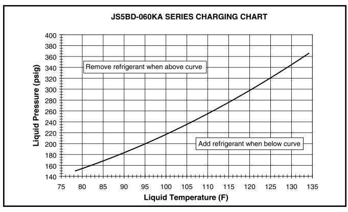
Figure 11. Charging Chart for 5 Ton Units
