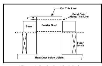
Figure 9. Feeder Duct Installation
