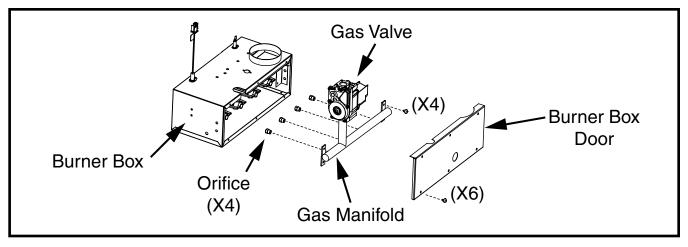
Figure 14. Orifice Removal
