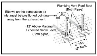
**Figure 4. Vertical Vent Termination**
