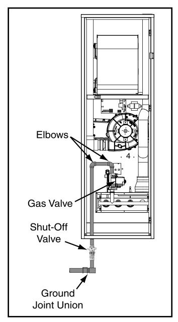
Figure 12. Typical Gas Connections
