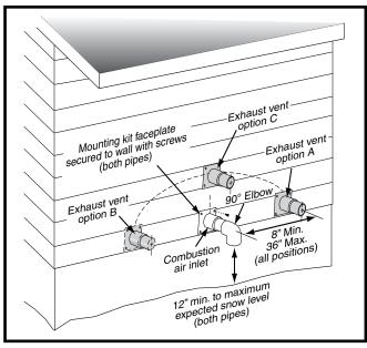
Figure 1. Inlet & Exhaust Pipe Clearances
