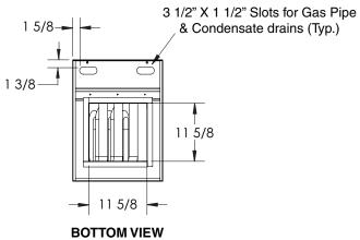
Figure 18. Furnace Dimensions
