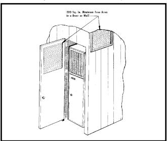
Figure 6. Closet Installation
