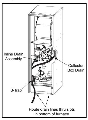
Figure 11. Condensate Drainage
