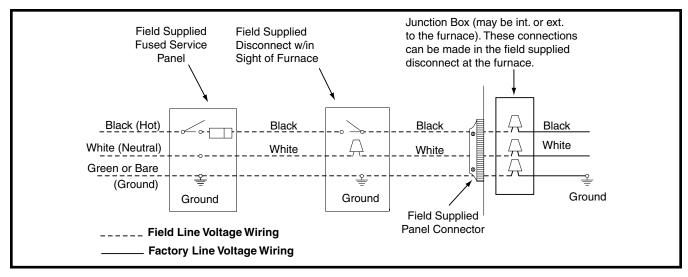
Figure 16. Line Voltage Field Wiring
