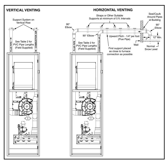
Figure 20. Horizontal & Vertical Venting
