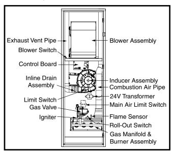
Figure 17. Furnace Components
