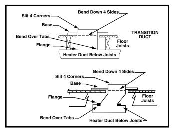
Figure 8. Transition & Offset Ducts
