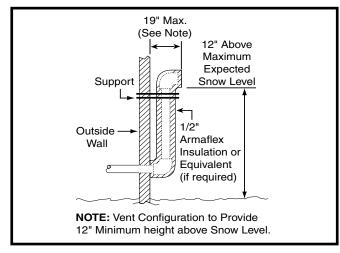
Figure 3. Alternate Horizontal Vent Installation
