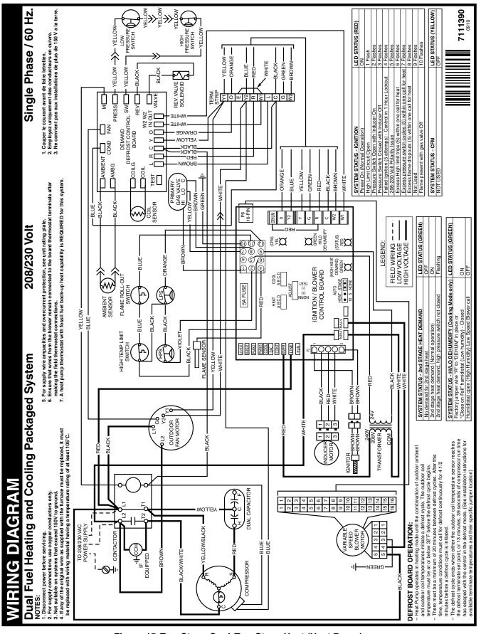
Figure 15. Two Stage Cool, Two Stage Heat (Heat Pump)
