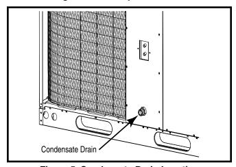
Figure 5. Condensate Drain Location
