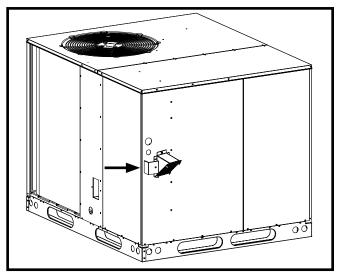
Figure 6. Ambient Sensor Location
