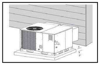
Figure 3. Ground Level Installation
