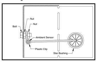
**Figure 7. Ambient Sensor Mounting**
