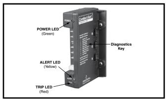
Figure 8. Comfort Alert™ Diagnostics Module
