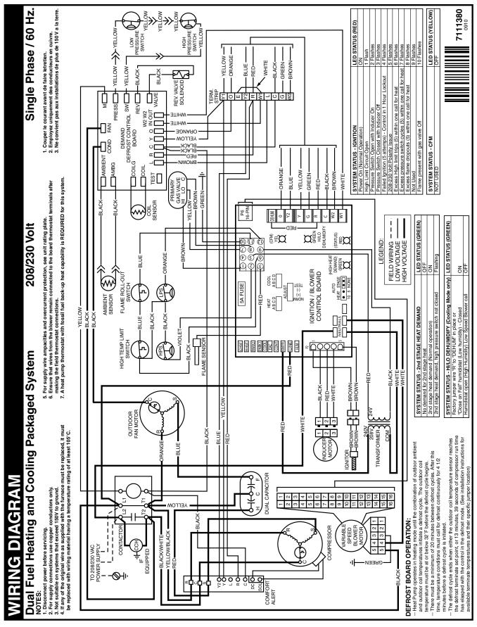
Figure 14. Two Stage Cool, Two Stage Heat (Heat Pump)
