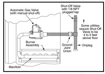
Figure 9. Typical Gas Hookup - Right Side Entry
