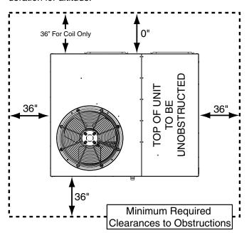
Figure 1. Clearance Requirements
