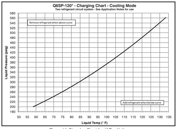
Figure 14. Charging Chart for 10 Ton Units
