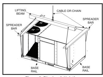
Figure 5. Rigging & Hoisting
