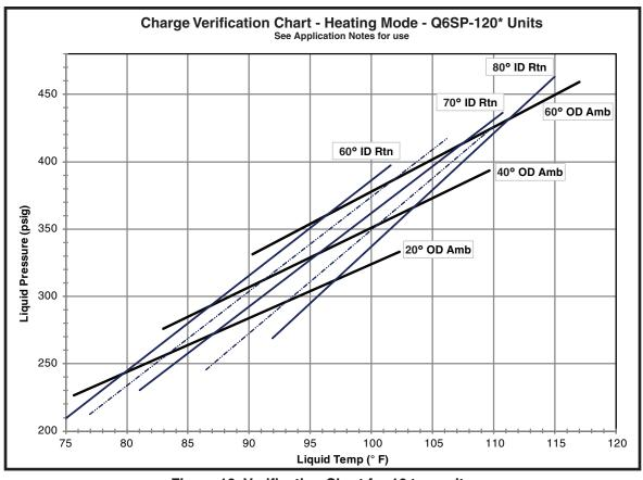
Figure 16. Verification Chart for 10 ton units
