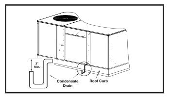
Figure 2. Condensate Drain
