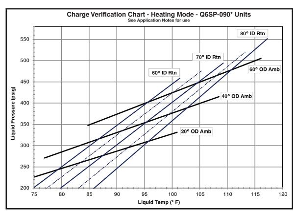
Figure 15. Verification Chart for 7 1/2 ton units
