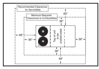
Figure 1. Minimum Clearances to Combustibles
