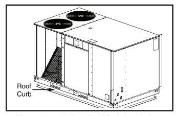
Figure 6. Installations Roof Curb Installations
