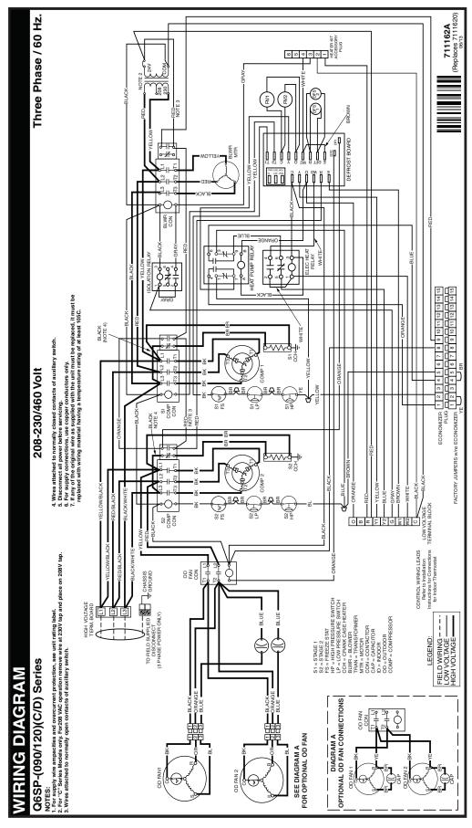
Figure 12. Wiring Diagram for Q6SP - 090/120 (C/D) Series
