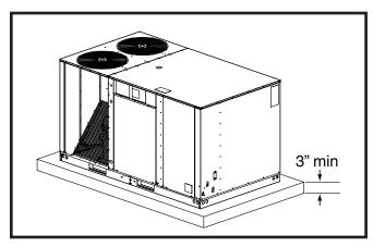
Figure 7. Concrete Pad
