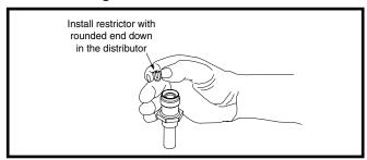
Figure 4. Restrictor Insertion into Distributor Body
