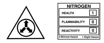
C8BA coils are pressurized with Nitrogen at the factory. Avoid direct face exposure or contact with valve when gas is escaping. Always ensure adequate ventilation is present during the depressurization process. Any uncertainties should be addressed before proceeding.
