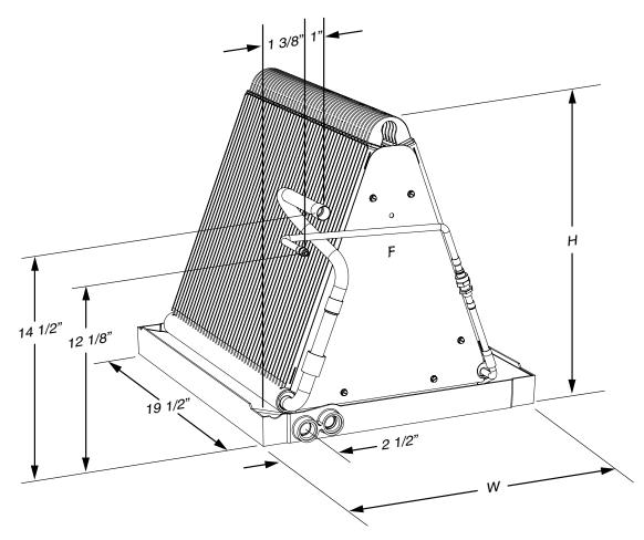
Figure 5. C8BA Coil Dimensions
