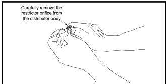
Figure 3. Removal of Orifice
