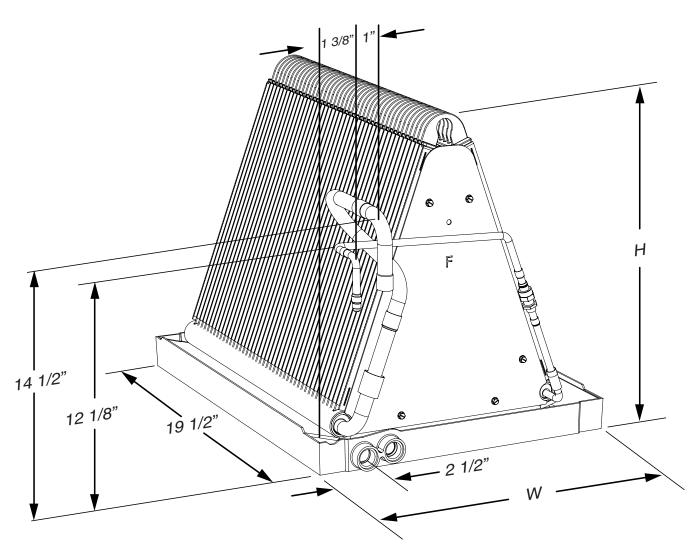
Figure 5. C8DA Coil Dimensions
