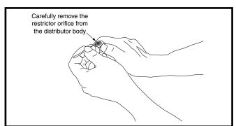
Figure 3. Removal of Orifice
