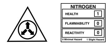
C8DA coils are pressurized with Nitrogen at the factory. Avoid direct face exposure or contact with valve when gas is escaping. Always ensure adequate ventilation is present during the depressurization process. Any uncertainties should be addressed before proceeding.
