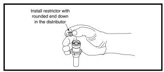
Figure 4. Restrictor Insertion into Distributor Body
