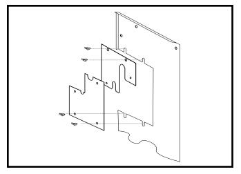
Figure 2. Close-Off Plate Assembly
