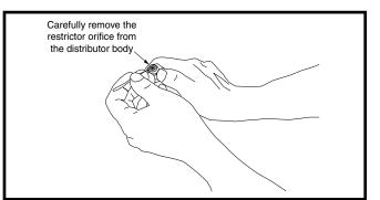
Figure 7. Removal of Orifice
