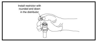
Figure 8. Restrictor Insertion into Distributor Body
