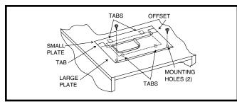
Figure 4. Close-Off Plates for Opening at Top of Furnace
