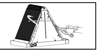
Figure 6. Loosening of Nut & Distributor Body
