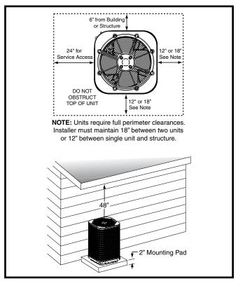
**Figure 1. Clearance Requirements**
