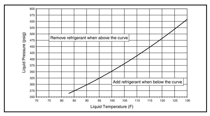
Figure 3. Charging Chart for S4BD-018 Series (1.5 Ton Units) - TXV Matches
