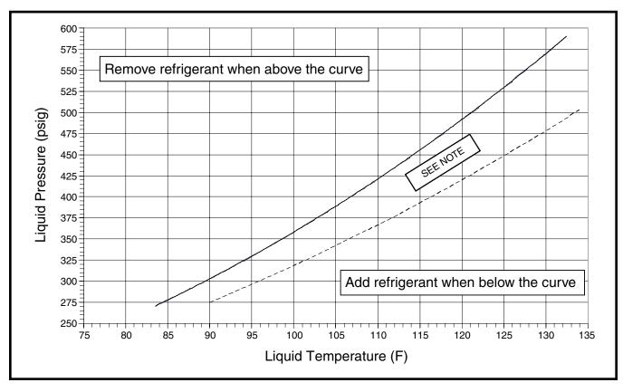
Figure 6. Charging Chart for S4BD-036 Series (3 Ton Units) - TXV Matches
