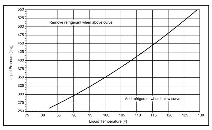
Figure 7. Charging Chart for T4BD-036 Series (3 Ton Units) - TXV Matches
