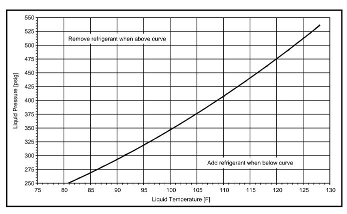
Figure 9. Charging Chart for T4BD-048 Series (4 Ton Units) - TXV Matches
