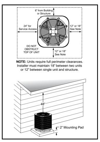
Figure 1. Clearance Requirements
