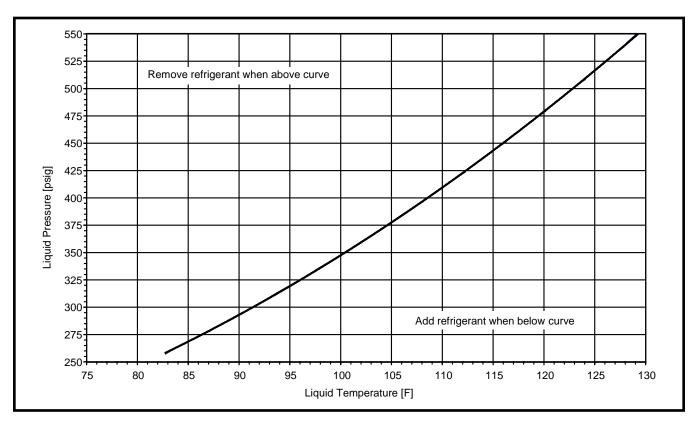
Figure 10. Charging Chart for T4BD-060 Series (5 Ton Units) - TXV Matches
