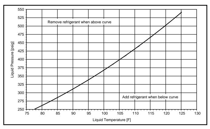
Figure 5. Charging Chart for T4BD-024 Series (2 Ton Units) - TXV Matches
