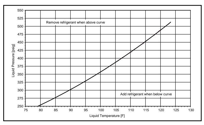
Figure 4. Charging Chart for T4BD-018 Series (1.5 Ton Units) - TXV Matches
