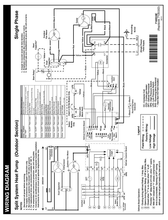
Figure 12. T4BD Wiring Diagram - Single Phase Models with Comfort Alert
