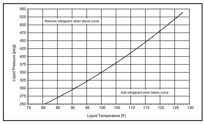
Figure 6. Charging Chart for T4BD-030 Series (2.5 Ton Units) - TXV Matches
