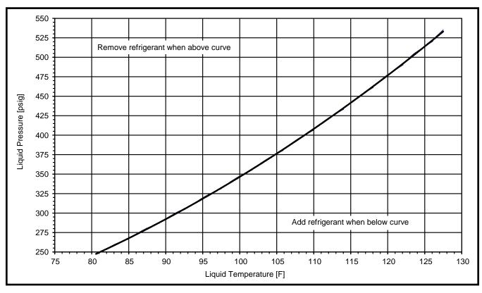
Figure 8. Charging Chart for T4BD-042 Series (3.5 Ton Units) - TXV Matches
