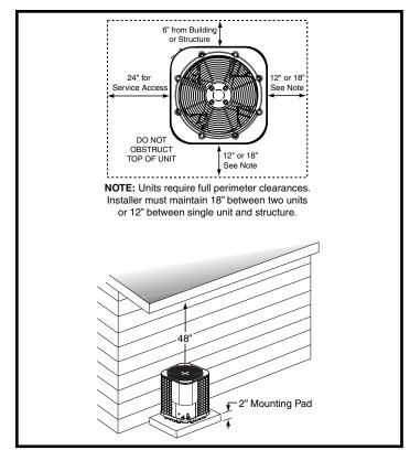
**Figure 1. Clearance Requirements**
