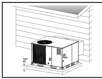
Figure 4. Ground Level Installation
