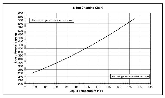
Figure 13. Charging Chart for 5 Ton Models (X60K Series)
