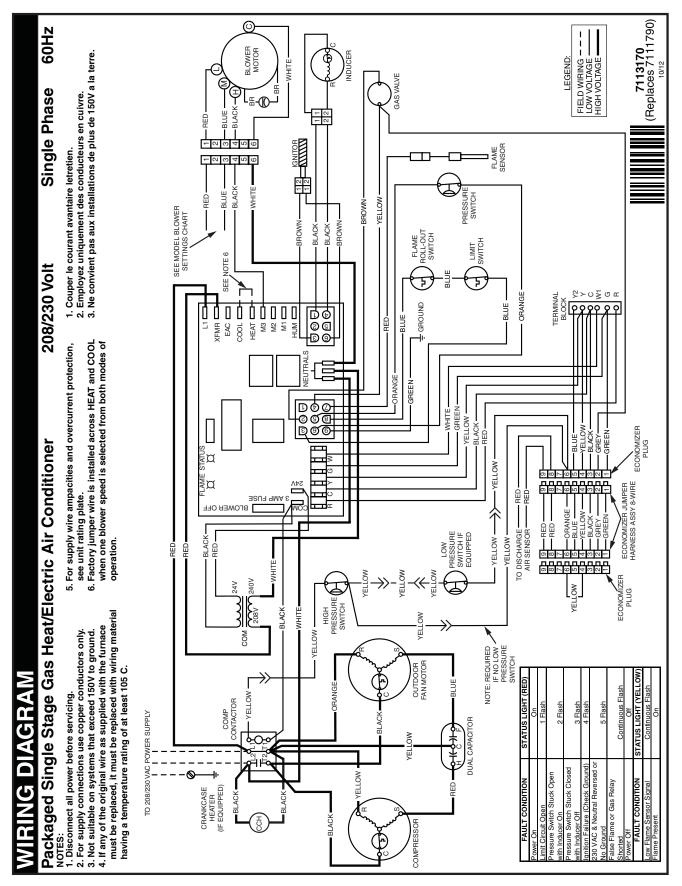
Figure 12. Wiring Diagram for 208/230V / 60 Hz Unit with PSC Motor
