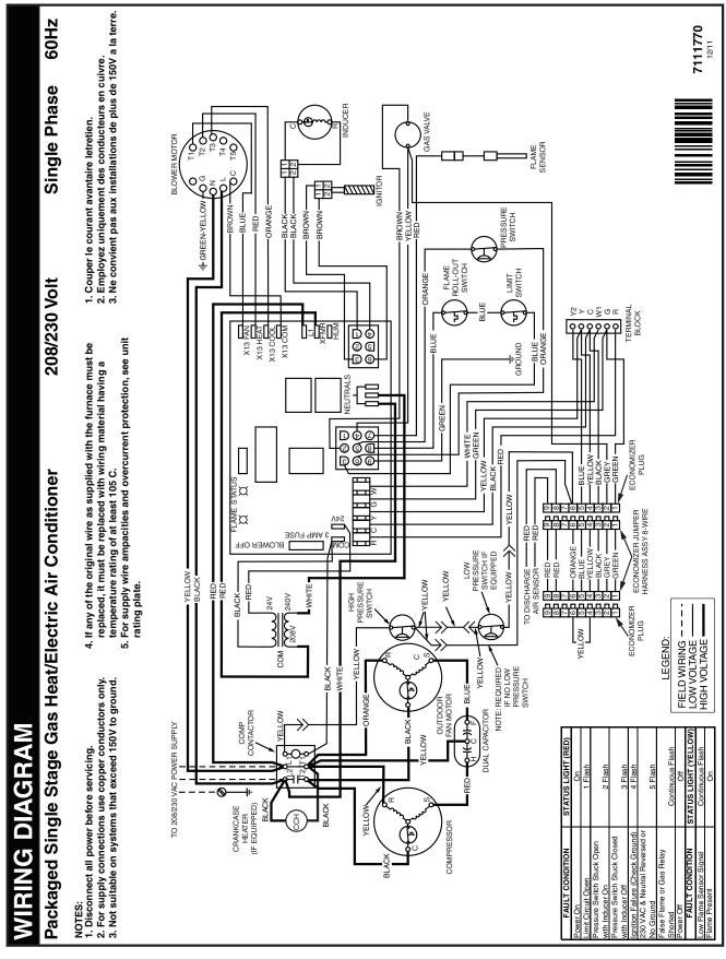
Figure 11. Wiring Diagram for 208/230V / 60 Hz Unit with ECM Motor
