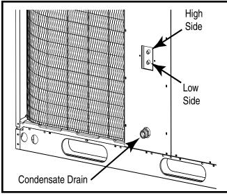
Figure 5. Refrigerant Service Ports & Condensate Drain Locations
