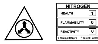
C7 coils are pressurized with Nitrogen at the factory. Avoid direct face exposure or contact with valve when gas is escaping. Always ensure adequate ventilation is present during the depressurization process. Any uncertainties should be addressed before proceeding.
