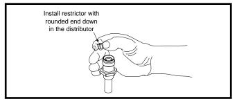
Figure 4. Restrictor Insertion into Distributor Body
