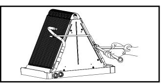
Figure 2. Loosening of Nut & Distributor Body
