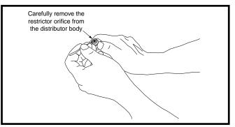
Figure 3. Removal of Orifice
