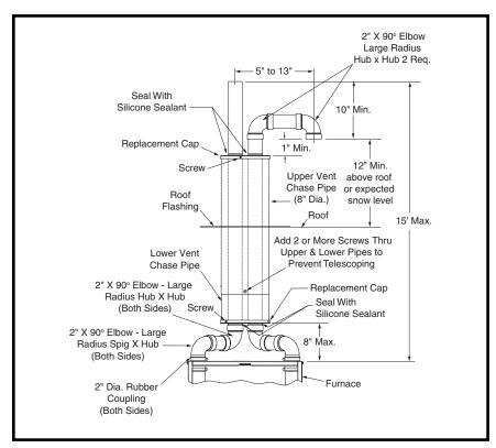
Figure 2. Vent & Combustion Air Intake Pipe Installation
