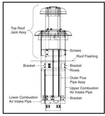
Figure 1. Typical Existing Roof Jack
